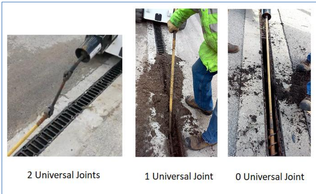
Figure 5.7. Different methods of attaching augers to HAB equipment
