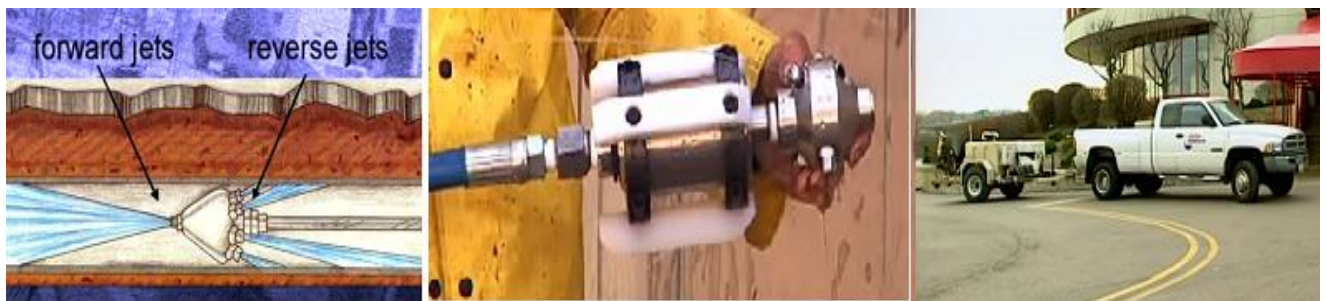
Figure 2.18. Cleaning a Trench Drain by a hydrojetter
