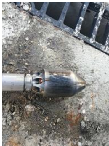
Figure 5.17. Modified Drainage Channel Nozzle
