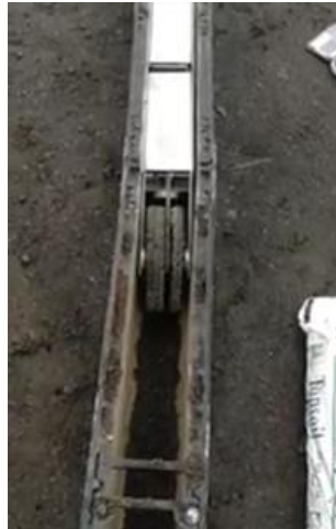
Figure 5.20. Test of UC cleaning robot with cutter assembly connected to Hurricane 500
