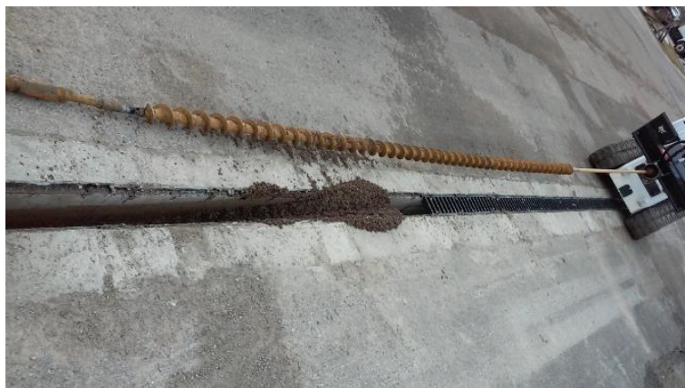
Figure 5.9. Testing set-up #3: no universal joint, 3 ¼ in. augers and front digger
