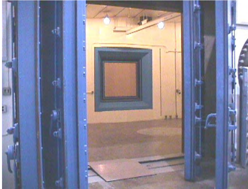
Figure 0.3: Entrance to the reverberation chamber showing the double noise reduction doors [provided by NASA Langley staff].
