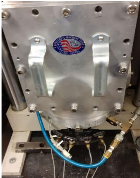
Figure 4.23. Closed chamber and drainage valves.
