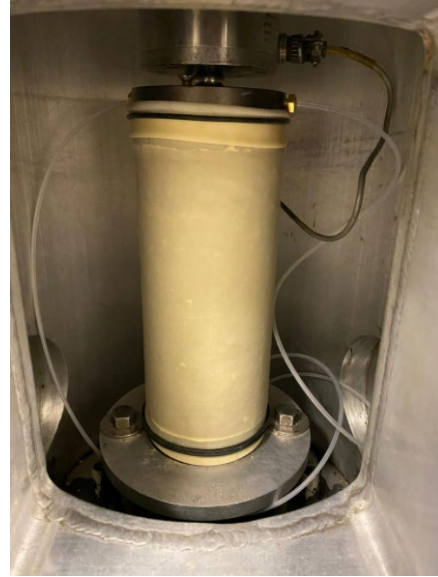
Figure 4.22. Sealed sample in triaxial chamber.
