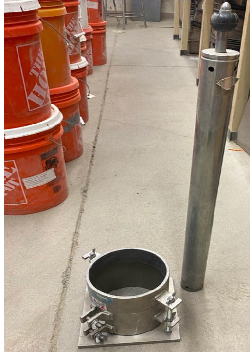
Figure 4.8. Modified Proctor equipment.
