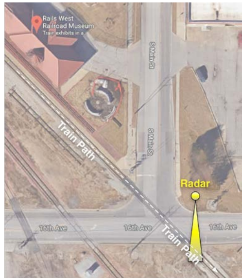
Figure 3.8 Field Test Configuration for Test03 . Note the 'Train Path' is actually opposite of what is shown above.
