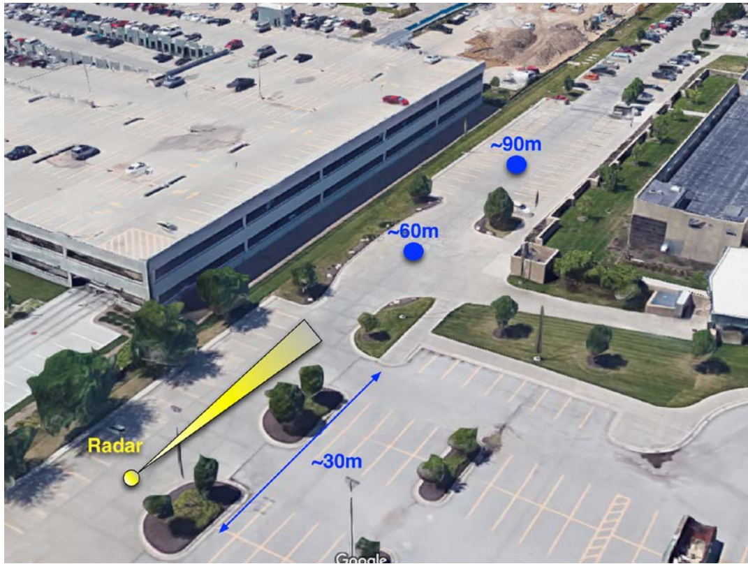
Figure 2.6 Parking Lot test setup with RADAR facing down straight parking lot section
