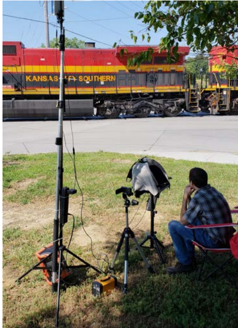
Figure 2.14 Radar Field testing setup while a locomotive passes by. Most of the time was spent waiting for trains. Here the train is departing from the Railroad Council Bluffs Yard with the train heading North-West, while the radar is pointed SOUTH across S. Main St.
