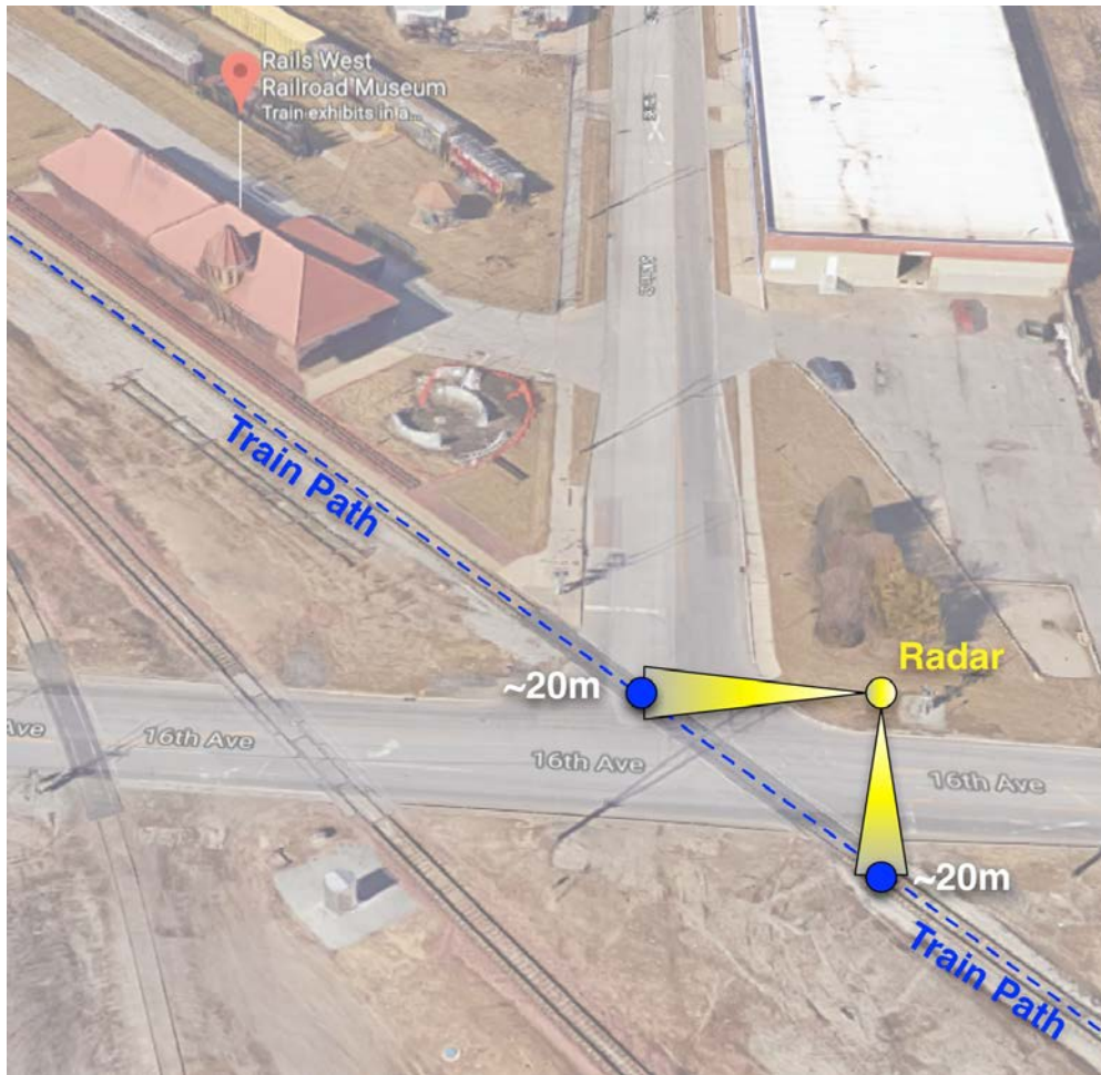
Figure 2.8 Slight side-view of the Rails West/Council Bluffs site radar configuration, showing radar placement, and main train path. There is a grade crossing at the intersection of 16 th Ave. and S. Main St.
