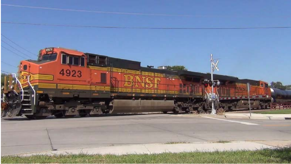
Figure 3.6 Initial set of locomotives, with sharp edges and rectangular nature provides a larger RCS to the radar.
