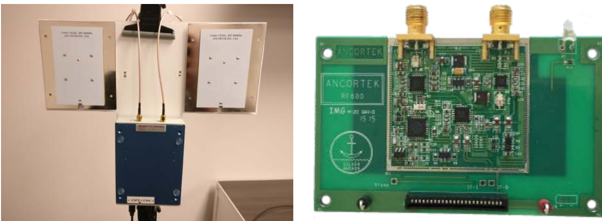
Figure 2.2 The SDRadar with its antenna setup (left), and the main system board (right)
