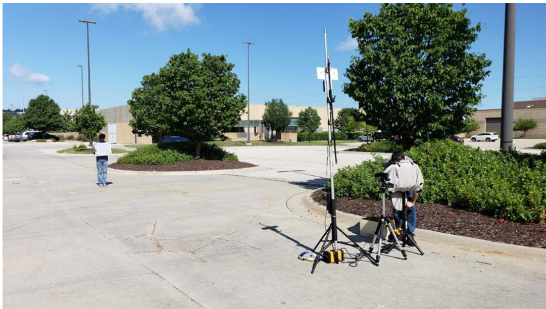
Figure 2.7 RADAR Reflector test used in pedestrian test scenarios
