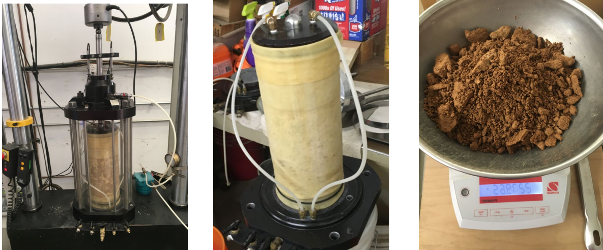
(a) RLT test (b) Specimen preparation (c) Scaling materials
