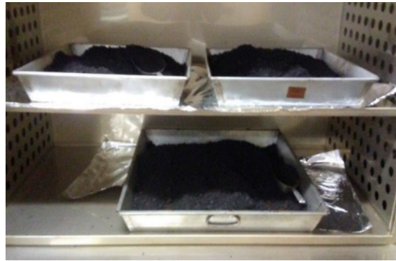
Figure 3.3 Heating the Asphalt Mix Inside an Oven at 165°C
