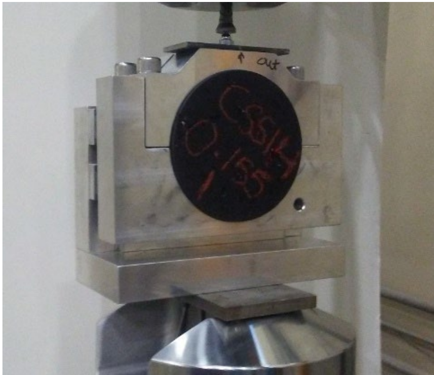
Figure 3.14 LISST Test in Progress
