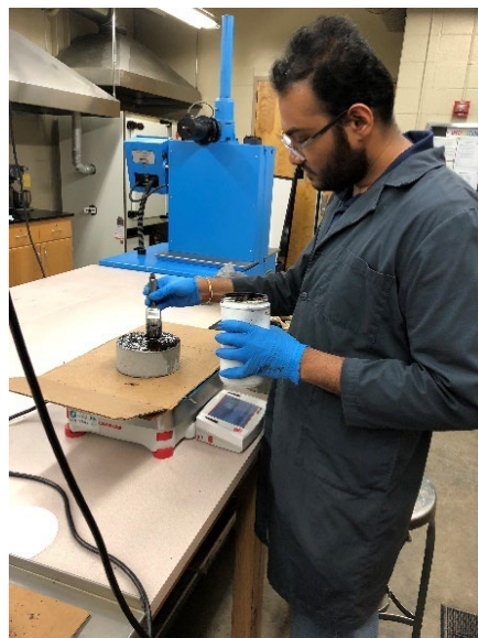
Figure 3.12 Applying Tack Coat on Bottom Layer Sample
