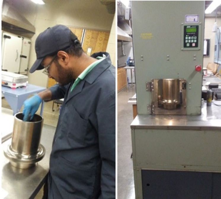
Figure 3.5 Preparation and Compaction of HMA Sample Using Superpave® Gyratory Compactor
