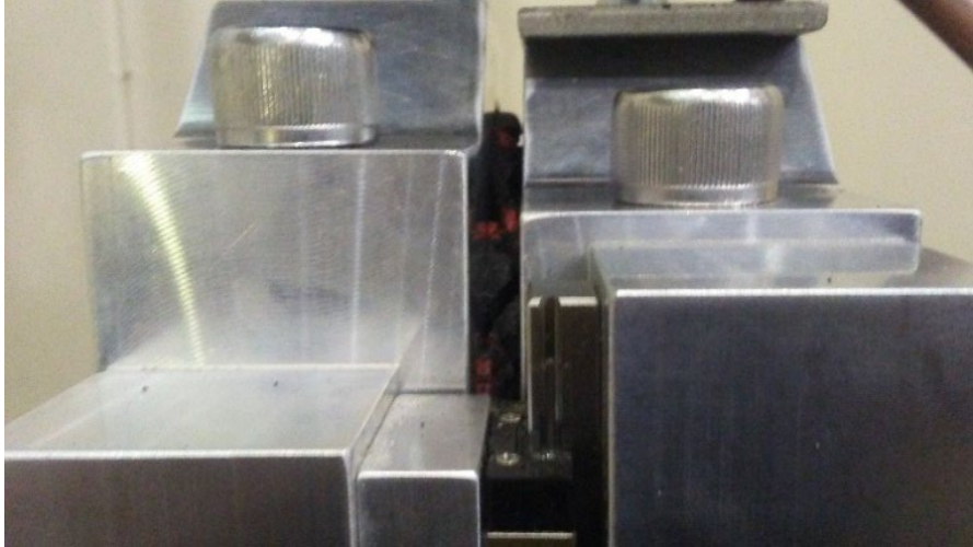
Figure 3.15 Interlayer Shear Failure in a Double-Layer Specimen
