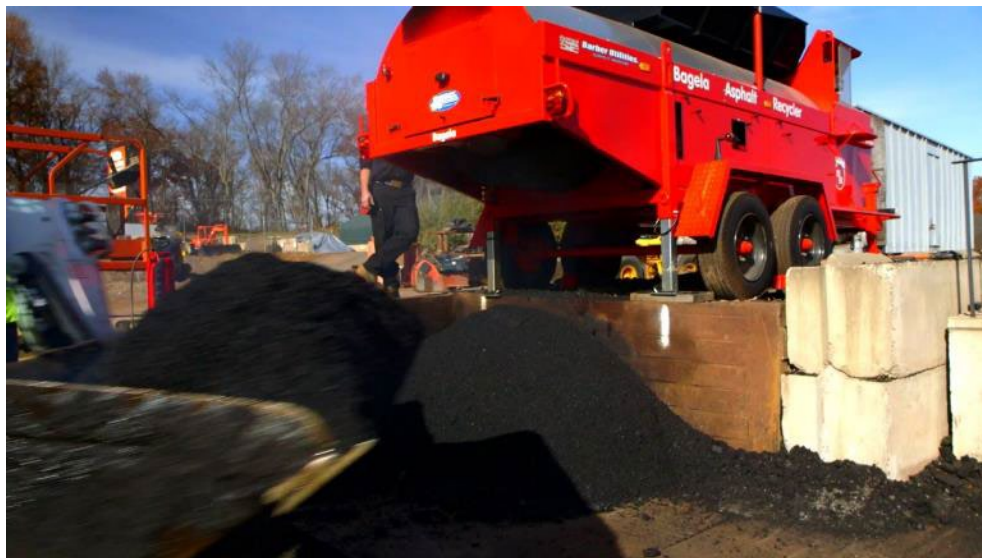
Figure B.8 Bagela recycler typically used by Ohio LPAs (Nazzal et al. 2020).
