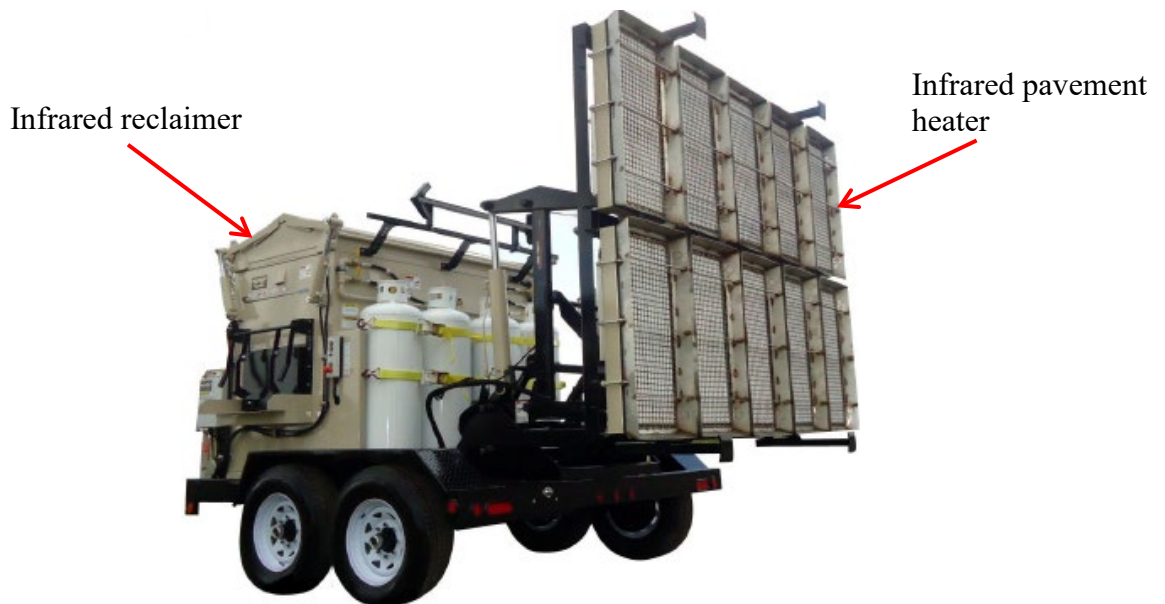
Figure B.9 Example of a tow-behind combination infrared asphalt heater/reclaimer
