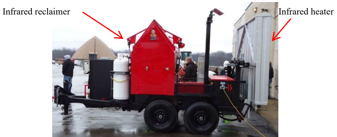
Figure B.6 An example of a tow-behind infrared asphalt heater/reclaimer
