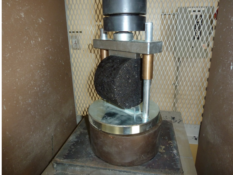
Figure 14. Specimen after Indirect Tensile Test
