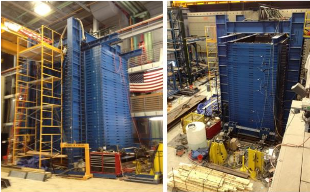
Figure 2-16 Laminar Shear Box and Hydraulic Actuators at the Base (Oakes, 2015)
