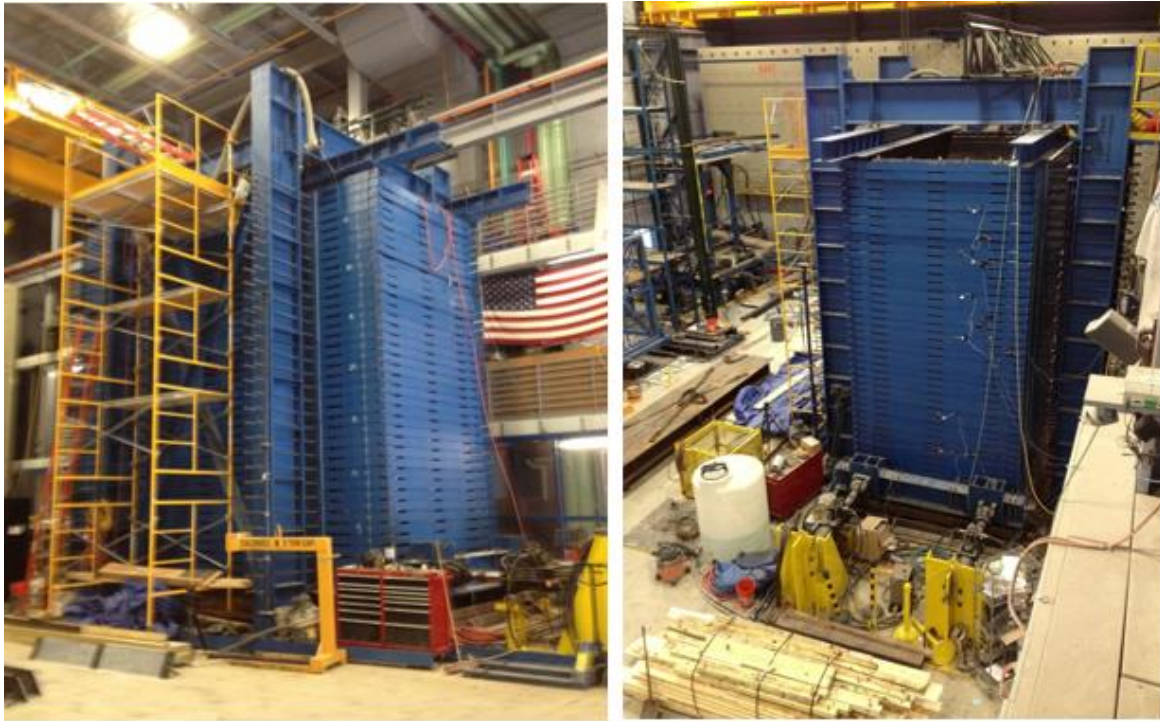
Figure 26 Photographs of the Laminar Shear Box and Hydraulic Actuators at the Base
