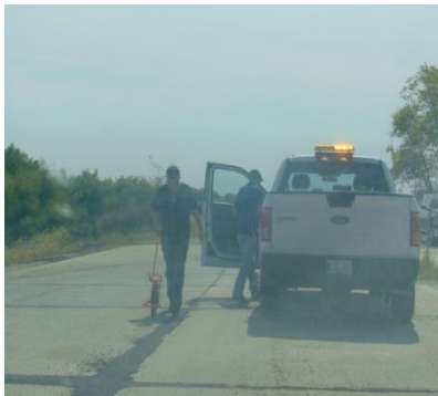
(a) Technician measures the distance to calibrate profilometer.
