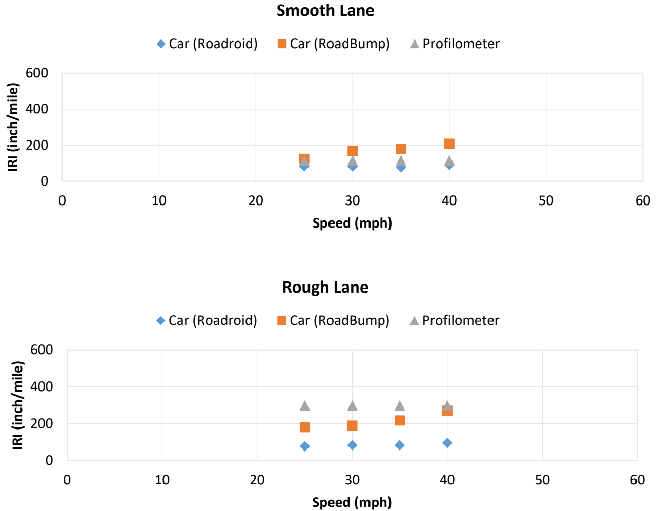
Figure 41. IRI values measured using a rolling profiler, and Roadroid and RoadBump apps.
