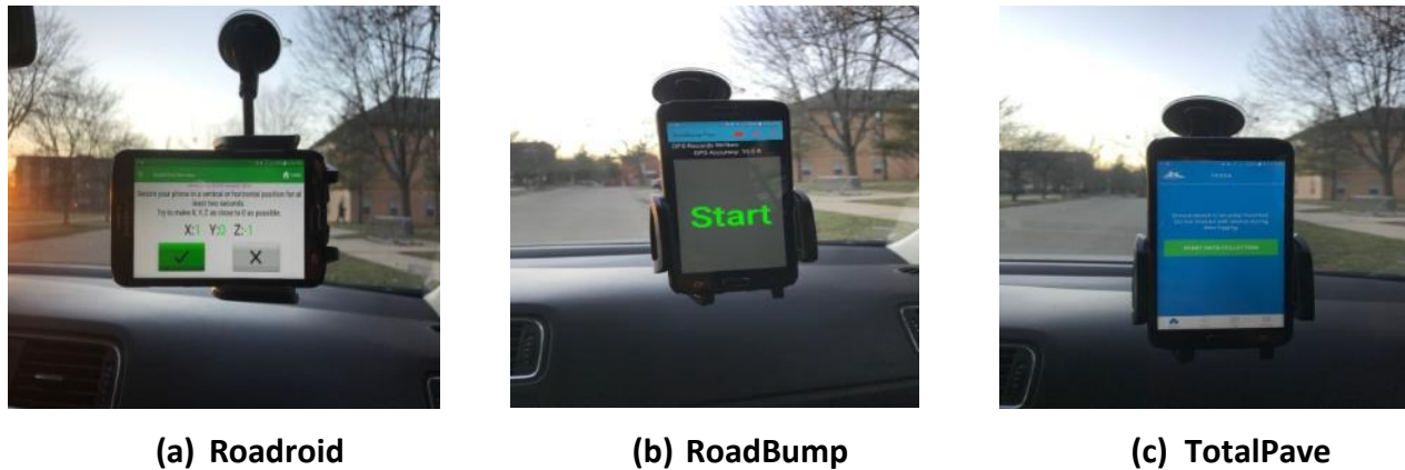
Figure C-14. Cell phone apps used to measure IRI of rural roads.
