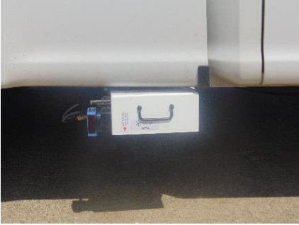
(b) Accelerometer and laser-beam source
