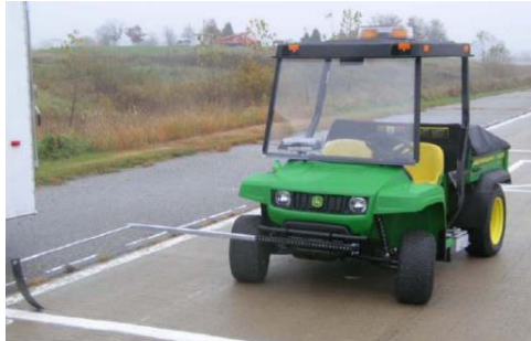
(a) Lightweight profilometer with the guidance system
