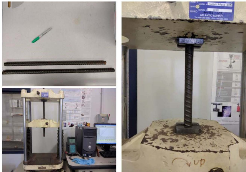
Figure 1-9 Reinforcing bar test.
