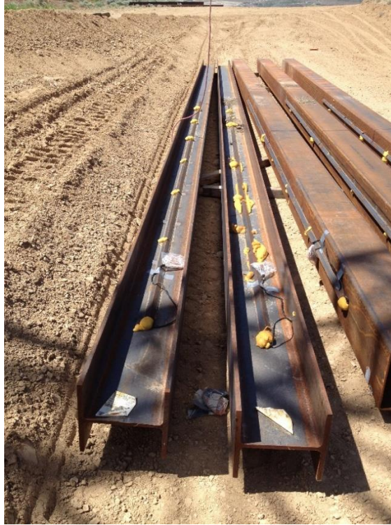
Figure 4-4: Strain Gauges Encased in a Steel Angle
