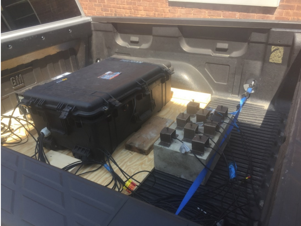
Figure 7.1 Pilot transport test AE equipment set-up
