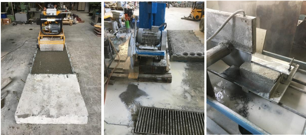
Figure 7. Preparation of RCC beam specimens.
