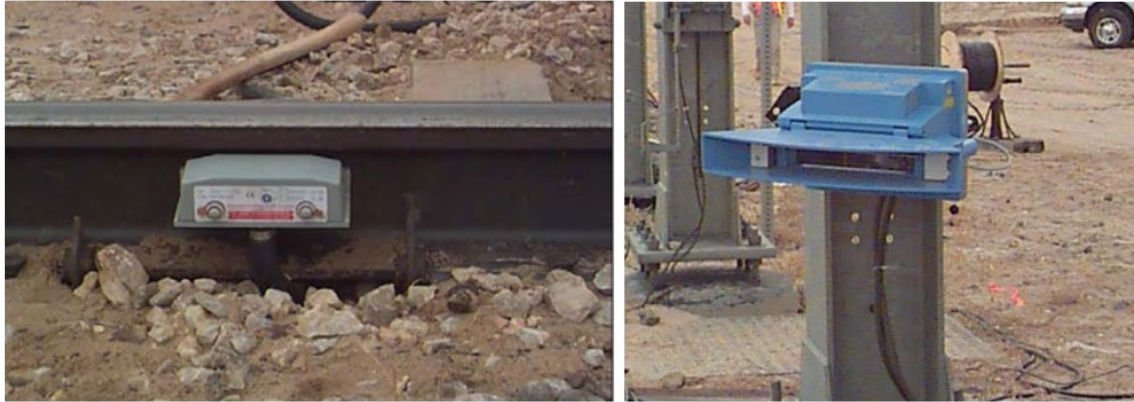
Figure 2.5 System 2 Wheel sensor (left) and vehicle/obstacle detection sensor (right) (Reiff et al. 2003)
