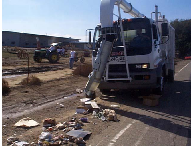
Figure 9.7 Automated Roadway Debris Vacuum [AHMCT, 2007].
