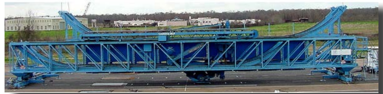
Figure 1 The accelerated wheel load test setup at the DOTD Pavement Research Facility
