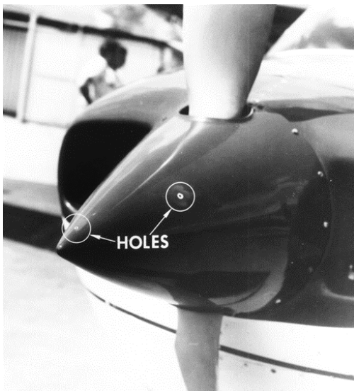
Fig. 4.27 Holes in aluminum spinner due to lightning attachments. (NASA photo).
