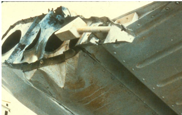
Fig 6.21 Result of exploded wire harness through fiberglass wing tip (gone) between navigation lamp and aluminum wing
