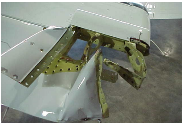
Fig 6.22 Result of inadequate bonding between navigation lamp and aluminum wing tip
