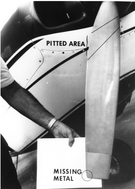
Fig. 4.26 Lightning strike damage to a metal propeller blade. This blade “cut through” the lightning channel after first being struck on its tip. The channel reattached to the inboard surface of the blade before the channel reattached further aft on the airplane. (NASA photo)
