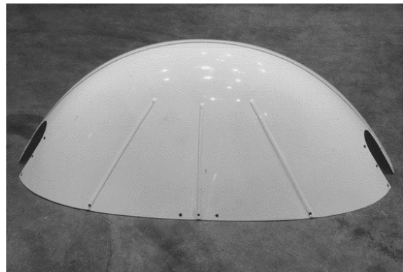
Fig. 6.28 Solid metal diverters on a radome.
