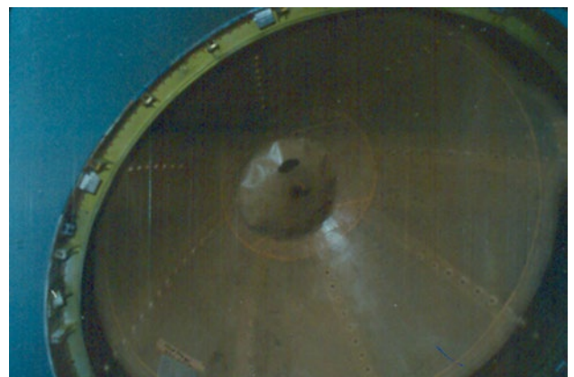
Fig. 4.20 Dis-bond of fiberglass sandwich inner surface due to streamer puncture.
