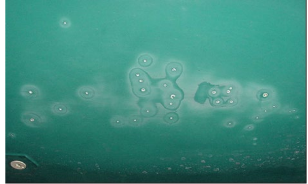
Fig. 4.8 Cluster of melted spots in painted aluminum fuselage skin. All are due to multiple reattachments in one strike. This cluster covers a region ~1 m in length along the lower fuselage of regional jet airplane. (Andy Plumer photo)
