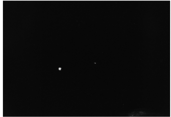
Fig. 7.35 Arcing at a bonded coupling. The larger spot of light is the optical fiber position light. The small spot is from arcing within the coupling.
