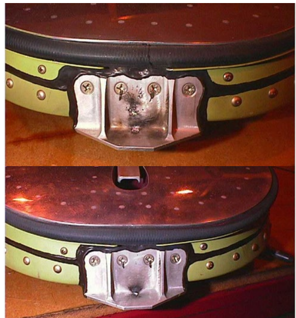
Fig. 4.10 Evidence of arcing at crew escape door stops during strike to door [4.2]
