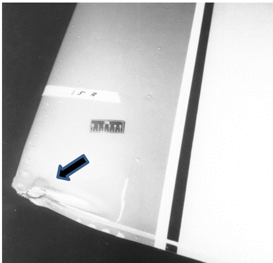
Fig. 4.9 Example of magnetic pinch effect at lightning attachment points. (NASA Photo)
