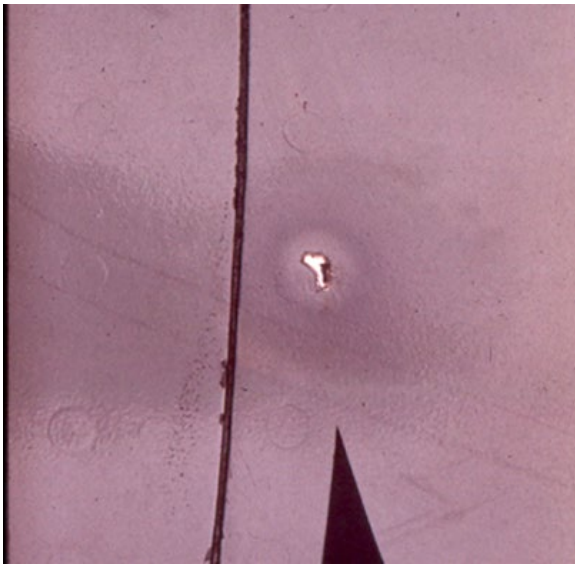
Fig. 4.7 Lightning channel reattachment to painted flush rivet. Note the thermal “halo” in the surrounding paint and darkening of paint aft (left) of the strike point. (Andy Plumer photo)
