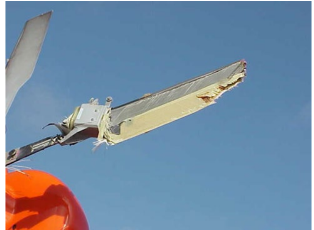
Fig. 4.29 Effects of lightning strike to a tail rotor (US Coast Guard Photo)
