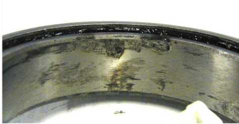
Fig. 4.11 Nose wheel axle and bearing after arcing due to lightning strike to nose wheel [4.2]
