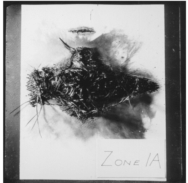
(a) Front side, showing thermal effects.
