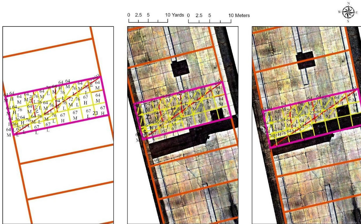
Figure 3. Manual Distress Survey Result (left); Manual Survey Results Overlaid on an RGB Data with Approximately 10-cm Position Accuracy (middle); and Well-aligned Manual Survey Results (right)
