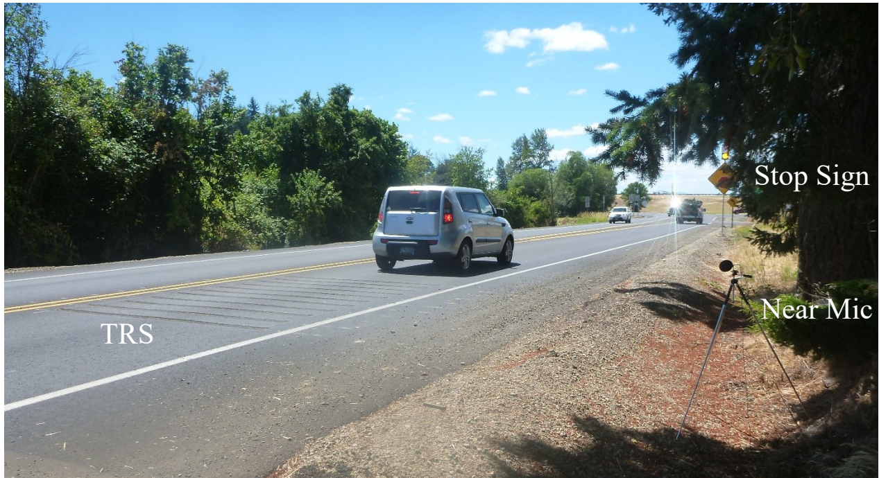
Figure 2.5: Before TRS roadside microphone setup
