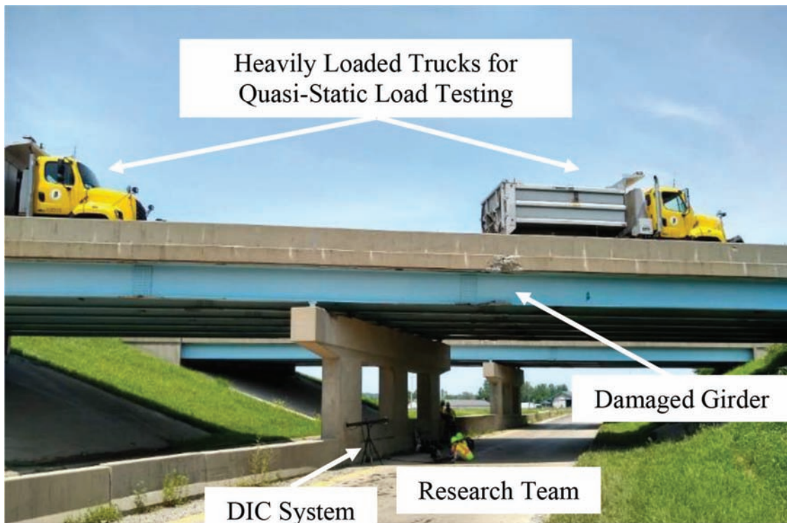
Figure 1.1 Field monitoring using DIC.
