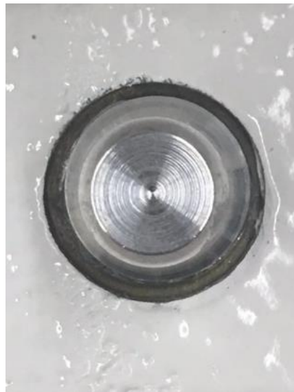
Figure 6. Pull Off Dolly (20 millimeter): Epoxied to Over Coated Steel Specimen
