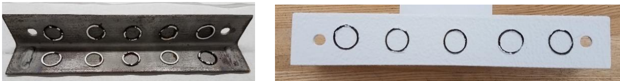
Figure 3. Specimen preparation: Attachment of O-rings using water soluble glue and their removal after the curing of the coating.
