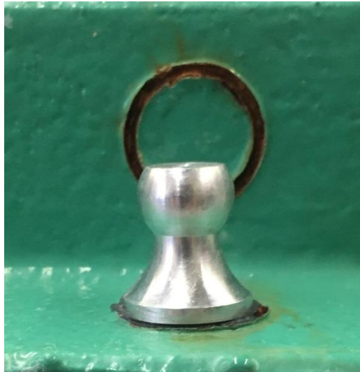
Figure 15. Pull Off Dolly (20 Millimeter): Epoxied to Inorganic Zinc Over Coated Steel Specimen
