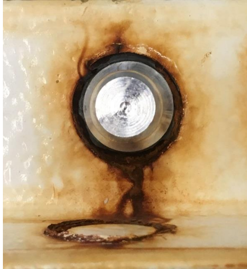
Figure 16. Pull Off Dolly (20 Millimeter): Epoxied to Epoxy Mastic Over Coated Steel Specimen
