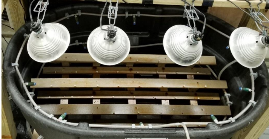
Figure 5. Chamber for Accelerate Testing: Salt Sprayers and Holding Rack
