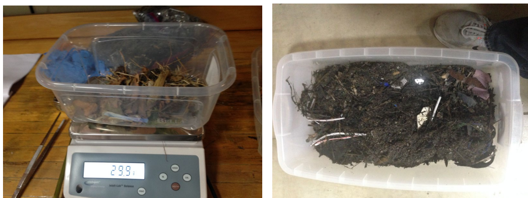
Figure 14. Examples of small (left) and large (bins) used to determine gross solids volume and mass.
