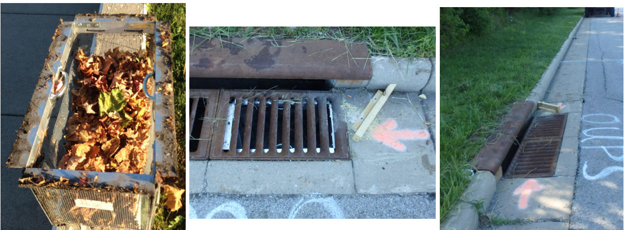
Figure 13. Gross solids monitoring equipment at field sites. Gross solids accumulated in the purpose-built catch basin insert at SR-48 (left), grate placed over catch basin insert at SR-49 (center), and wooden diverter in gutter pan at SR-49 (right).
