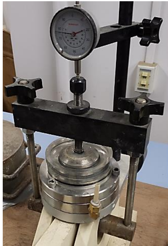
Figure 5-8 Fully assembled cell in table top oedometer.
