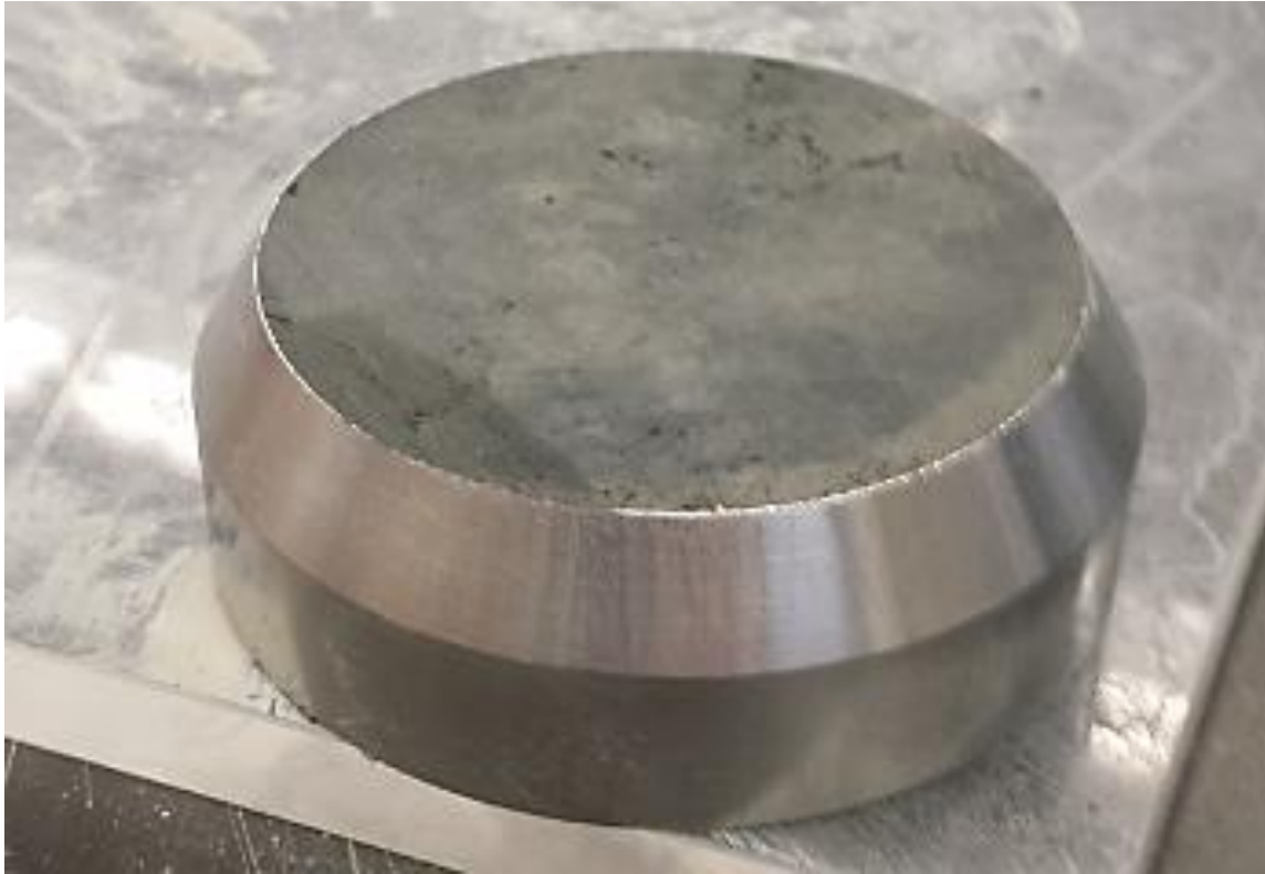
Figure 5-6 Sample in consolidation ring
