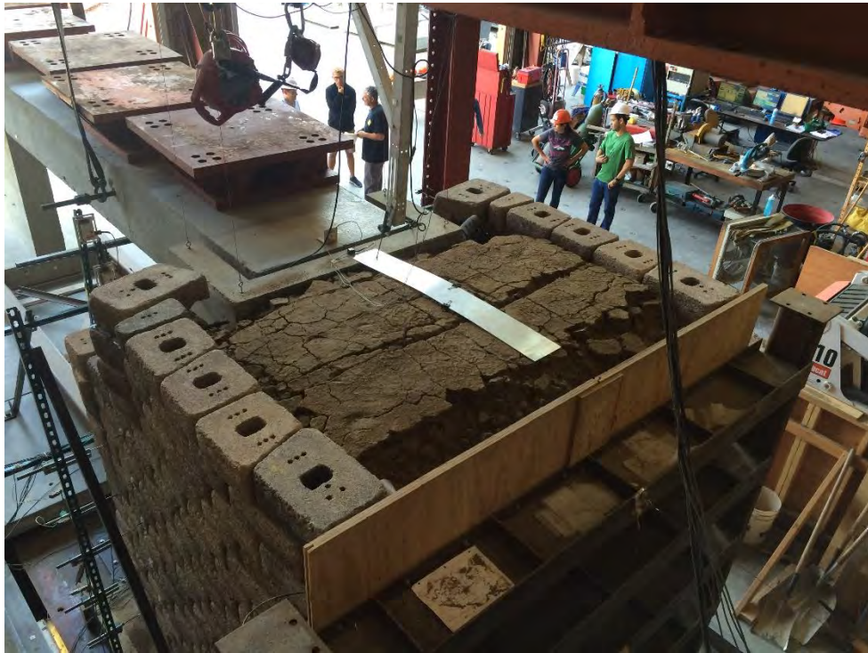
Figure A2.40 Top view after all shaking motions for Test 3.
