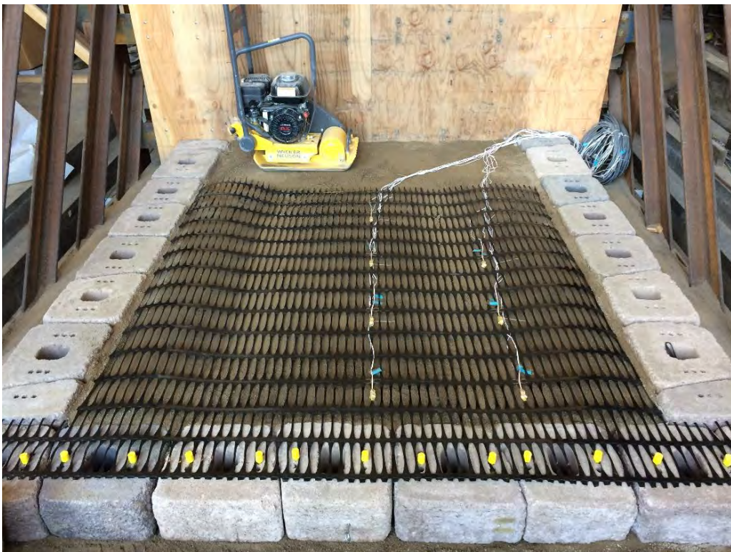
Figure A2.4 Longitudinal reinforcement layer.
