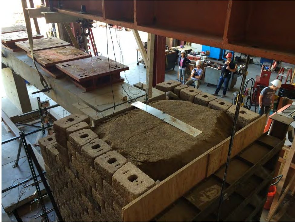
Figure A2.47 Top view after the Northridge motion for Test 5.
