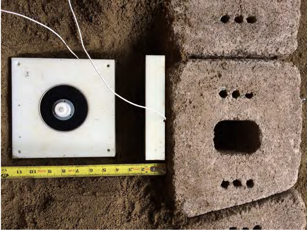
Figure A2.9 Total pressure cells placed behind wall facing.
