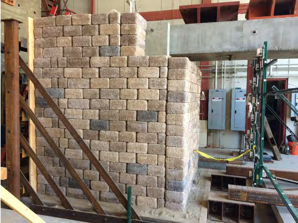
Figure A2.21 Constructed specimen for Test 1.
