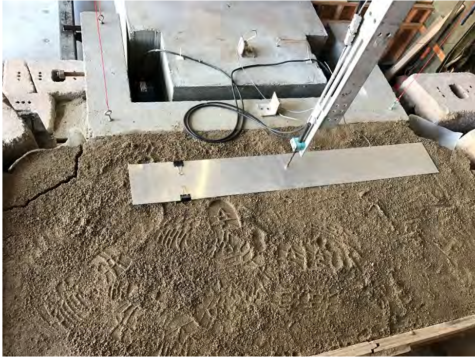
Figure A2.49 Upper wall backfill surface after the Maule motion for Test 6.
