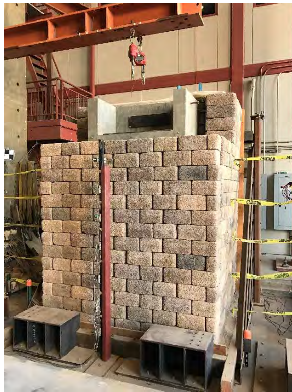
Figure A2.30 Constructed specimen for Test 6.
