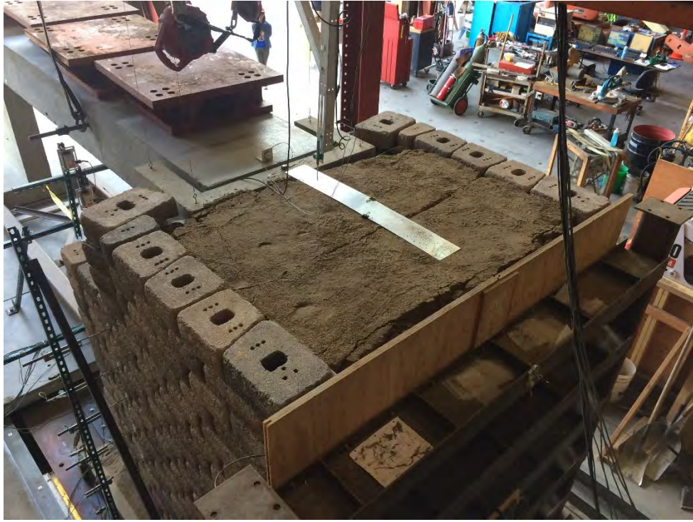
Figure A2.39 Top view after the Northridge motion for Test 3.
