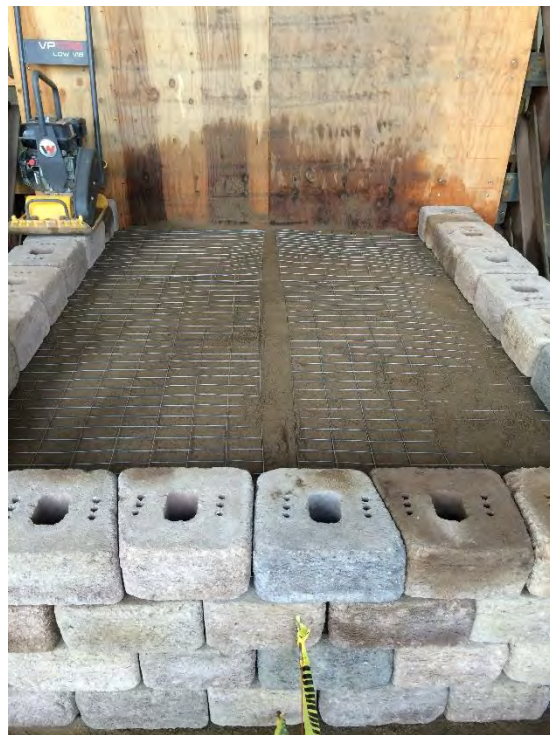
Figure A2.6 Transverse reinforcement layers for Test 5.
