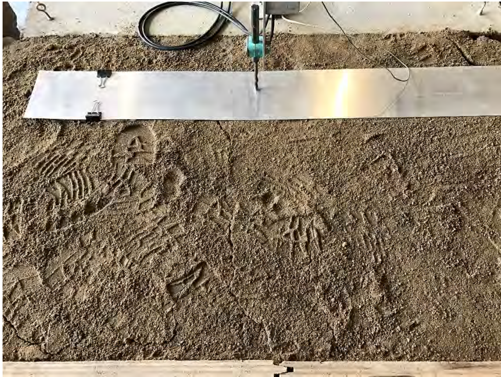
Figure A2.50 Minor crack after the Northridge motion for Test 6.
