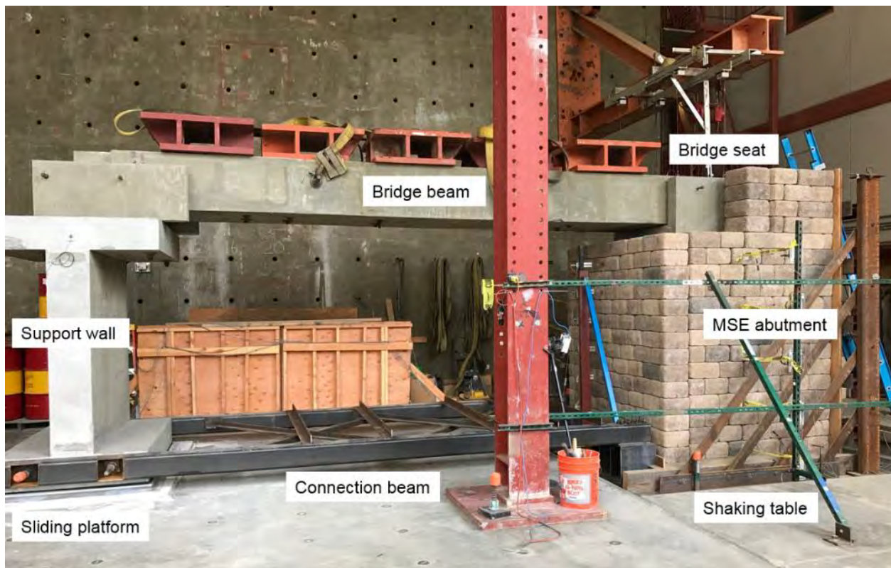
Figure 3.20 Shaking table test configuration of bridge system for the transverse test.
