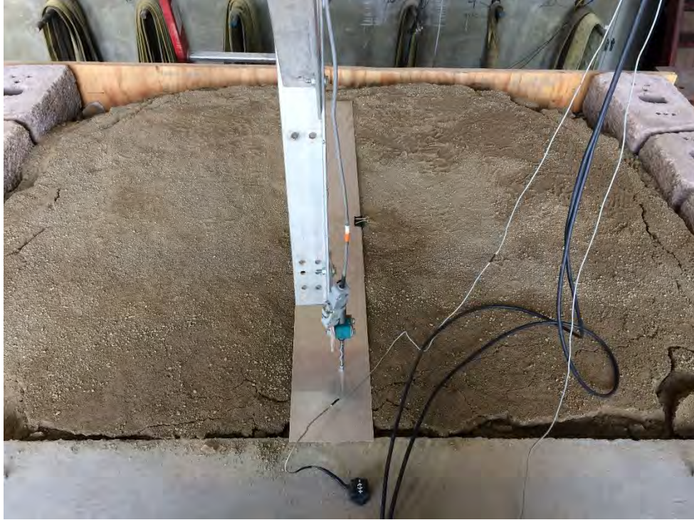
Figure A2.35 Upper wall backfill surface after all shaking motions for Test 1.
