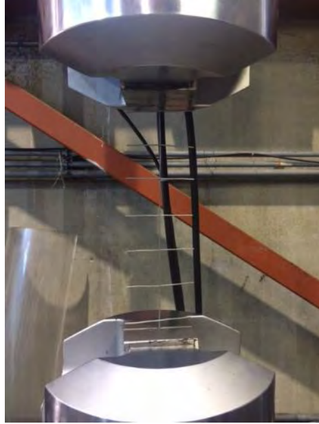
Figure 3.15 Tensile test on steel welded wire mesh.
