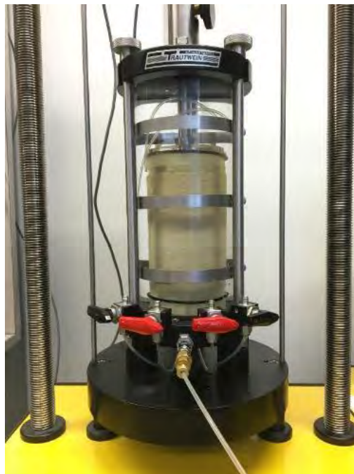
Figure 3.7 Consolidated drained triaxial compression test setup.
