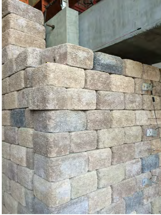
Figure A2.41 Movements of the top corner blocks after all shaking motions for Test 3.
