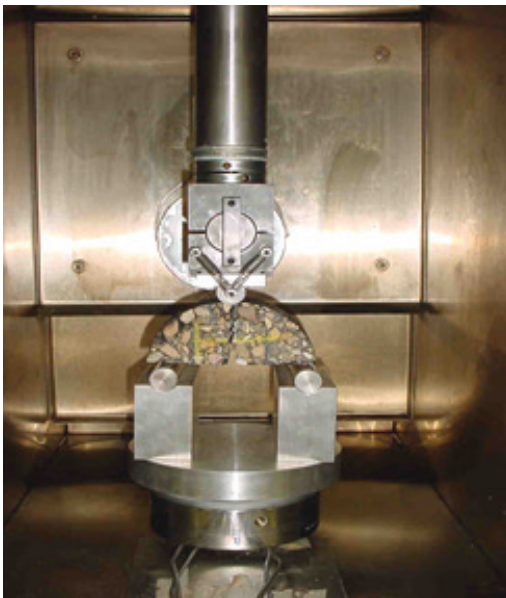
Figure 2 SCB test setup
