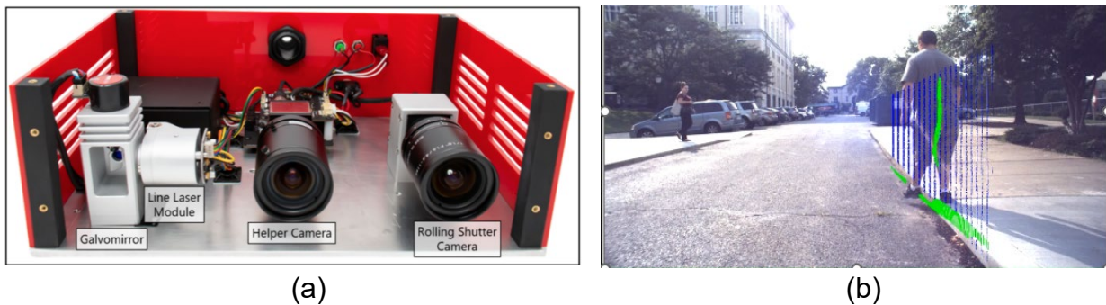
Figure 14: (a) Programmable Light Curtain (PLC) sensor; (b) PLC detection of pedestrian movement from the sidewalk into the street.
