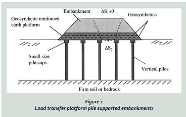
embankment on soft clay soil to improve the soil's ability to carry the applied load.
