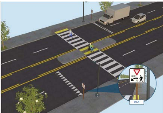
Advance yield here to pedestrian sign and yield line (Federal Highway Administration 2020b)
