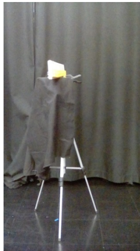
Figure 29. Yellow delineator sample mounted on tripod
