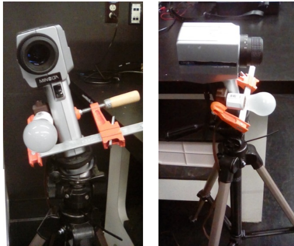
Figure 27. Luminance meter and light source (left: front view, right: side view)
