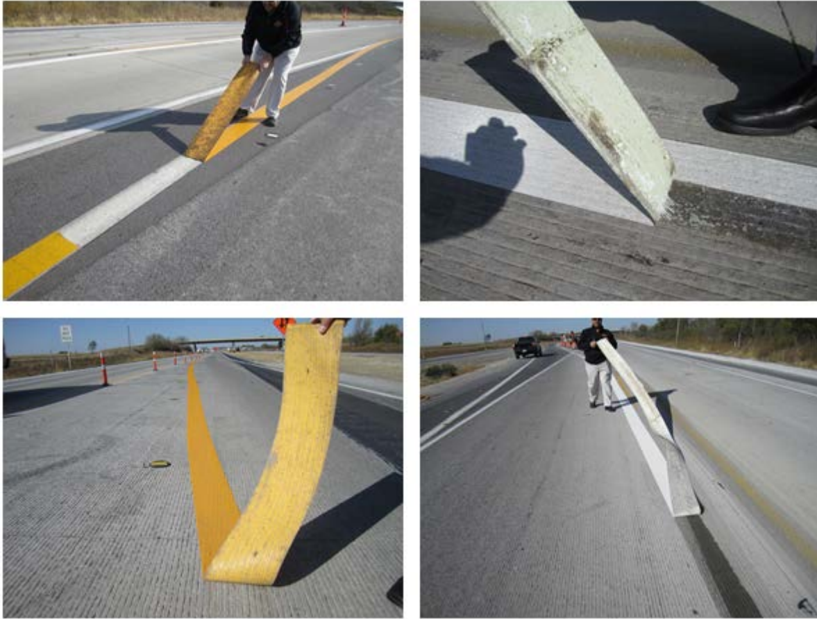
Figure 18. Variety in effort required to remove tape products
