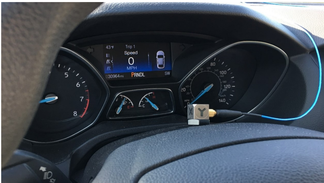
Figure 4.10: Accelerometer placement in passenger car
