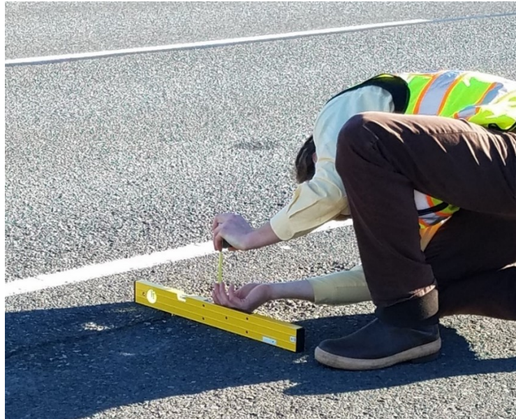
Figure 4.25: Measuring the depth of an individual mill
