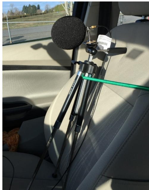
Figure 4.12: Microphone placement in passenger car
