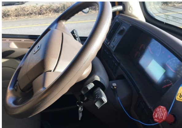
Figure 4.20: Accelerometer placement in heavy vehicle
