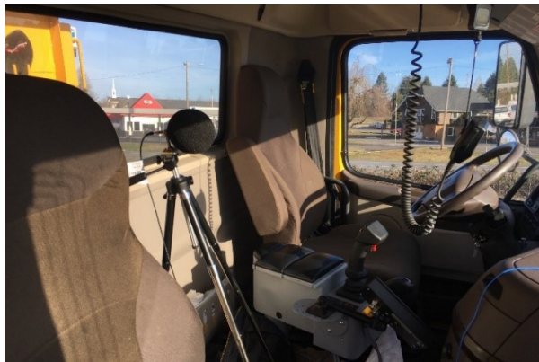
Figure 4.21: Microphone placement in heavy vehicle
