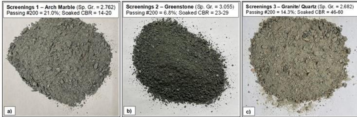
Figure 3. No. 10 Screenings: a) screening 1; b) screening 2; c) screening 3. Sp. Gr. = specific gravity; CBR = California bearing ratio.
