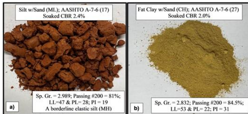
Figure 2. Subgrade Soils: (a) silt (borderline elastic) from Lynchburg; (b) fat clay from Fairfax. Sp. Gr. = specific gravity; LL= liquid limit; PL = plastic limit; PI = plasticity index; CBR = California bearing ratio.
