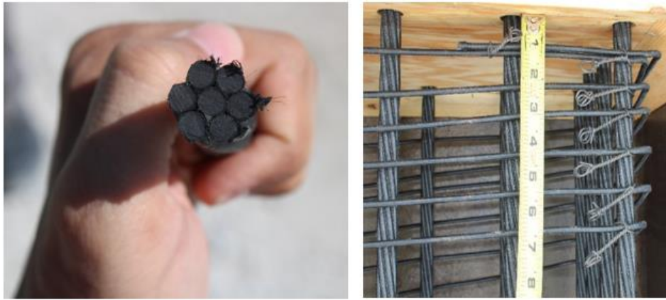
Figure E3: The CFRP strands and spirals used for the construction
