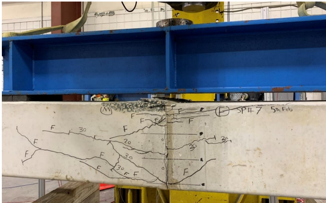
Figure 103: Crack propagation and failure mode of Specimen 7
