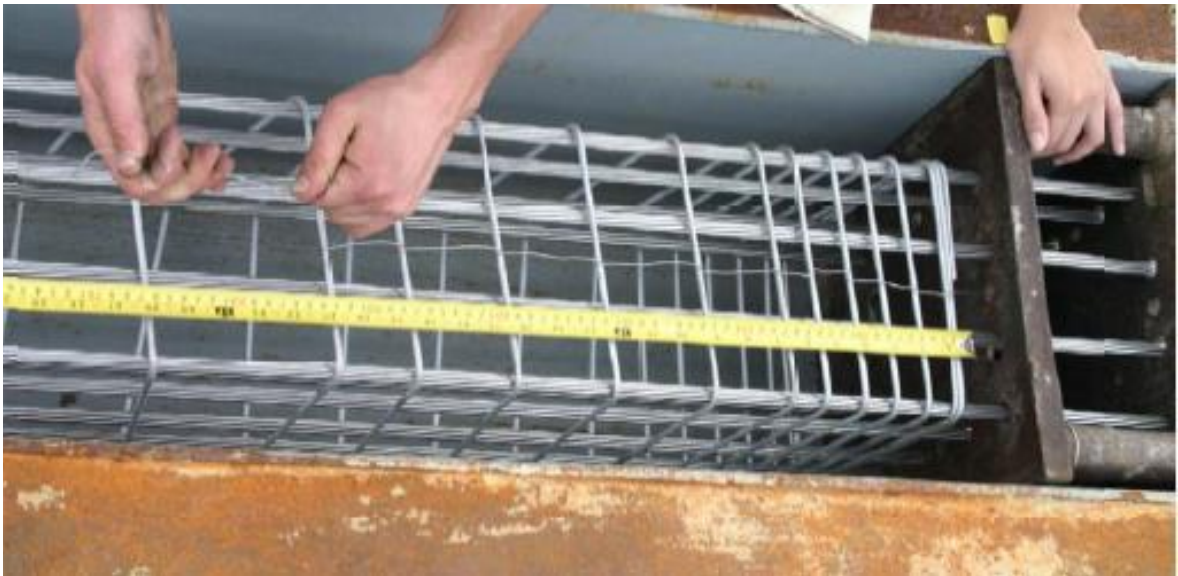
Figure 11: PPCP with stainless steel strand and spiral [26]
