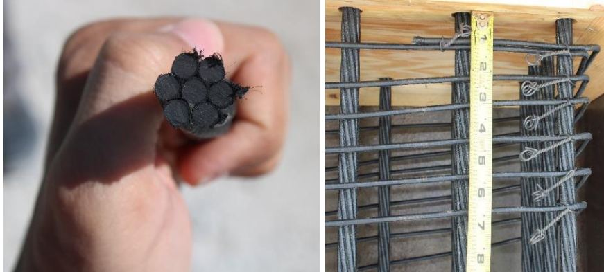
Figure 49: The CFRP strands and spirals used for the construction
