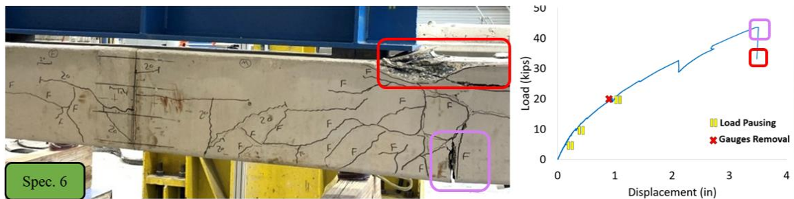
Figure 126: Failure mode of flexural cracking – debonding in the male Specimen 6
