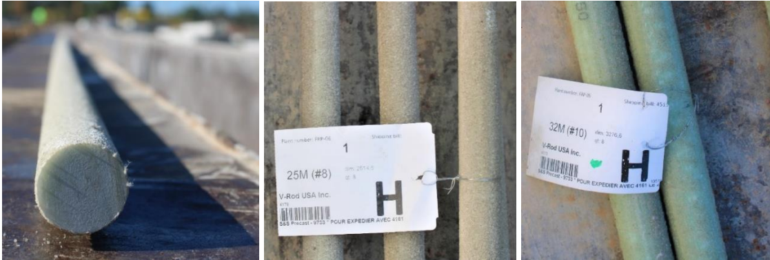
Figure 48: The GFRP bars used for the construction
