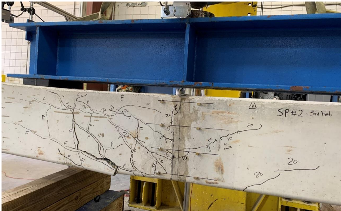
Figure 77: Crack propagation and failure mode of Specimen 2
