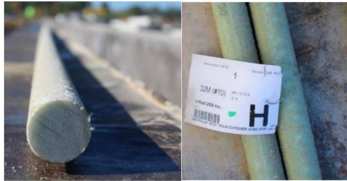
Figure E2: The GFRP bars used for the construction of PPCP splicing
