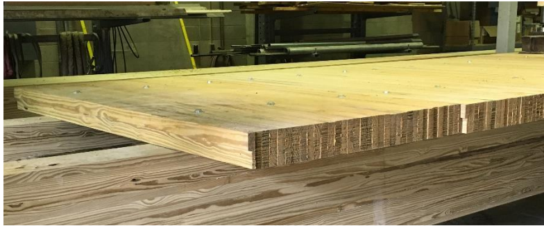
Figure 25. Lap splice edges on glulam deck panels for Large-Scale Specimens 1 and 2
