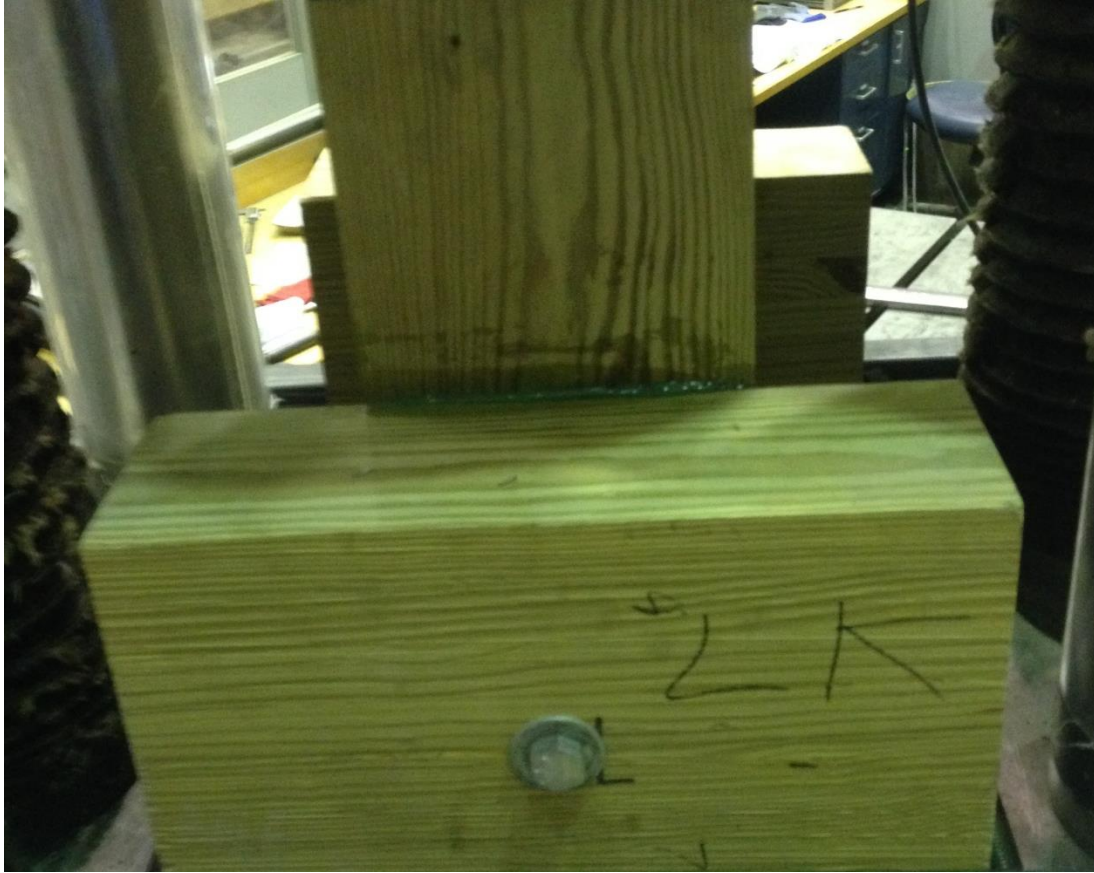
Figure 20. Small-scale specimen with epoxy and lag screws
