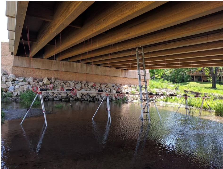
Figure 34. Typical instrumentation setup for testing of the composite timber bridge
