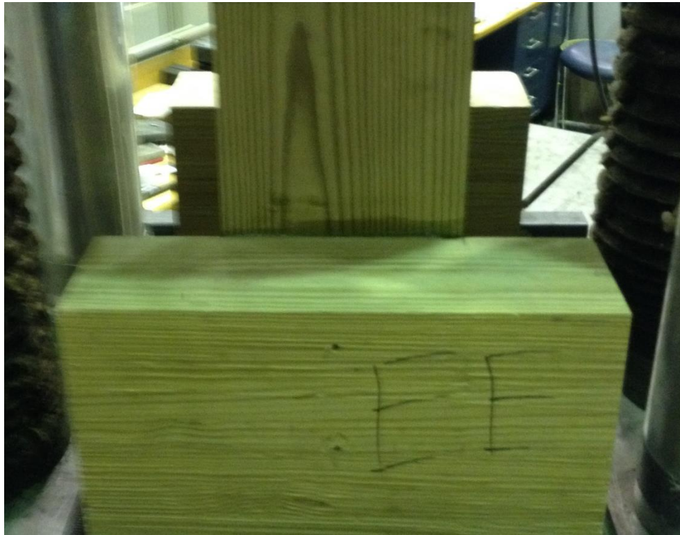
Figure 22. Small-scale specimen with epoxy and GRK screws removed
