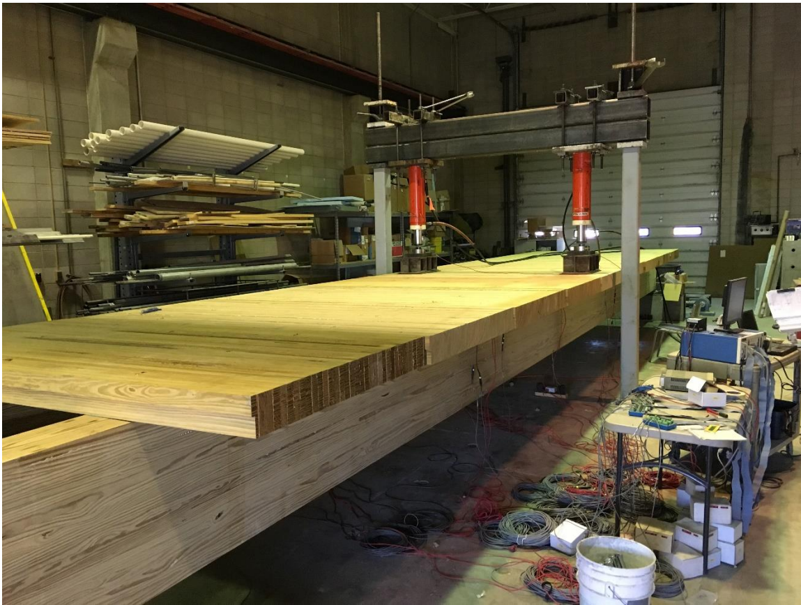
Figure 29. Installation of glulam deck sections on Large-Scale Specimen 2 using epoxy
