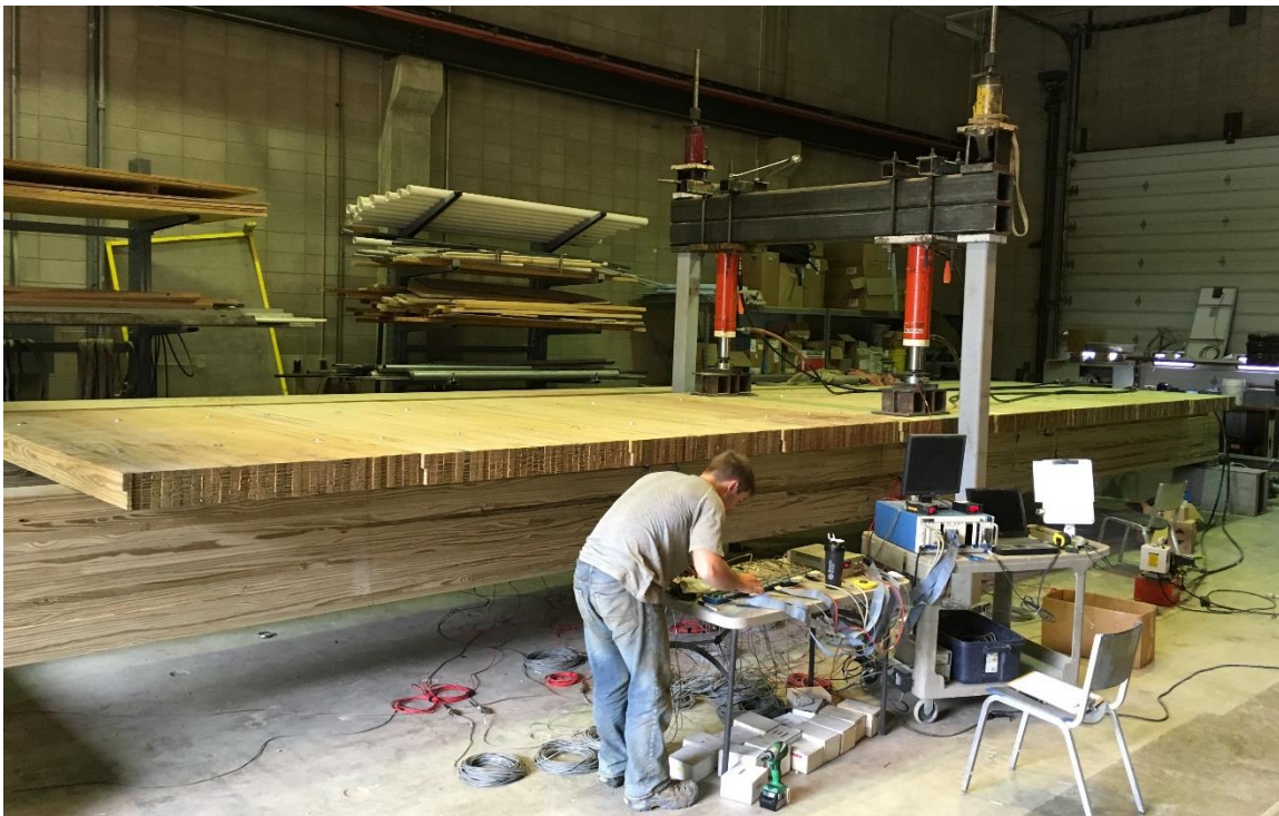
(b) Large-Scale Specimen 1 erected and being prepped for testing
