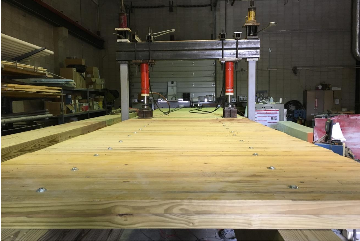
(a) Glulam deck panels lag-screwed to girders on Large-Scale Specimen 1
