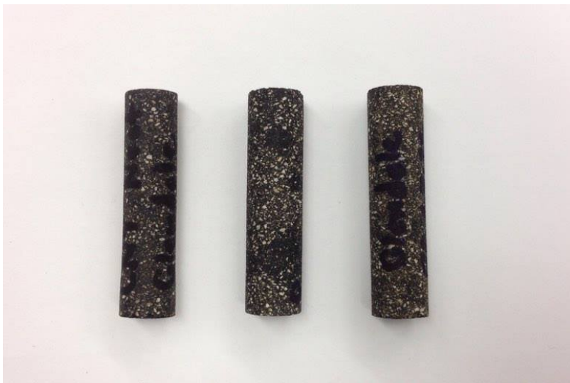
Figure 4.2. Typical FAM Test Specimens Cored Out of a Superpave Gyratory Compacted Specimen
