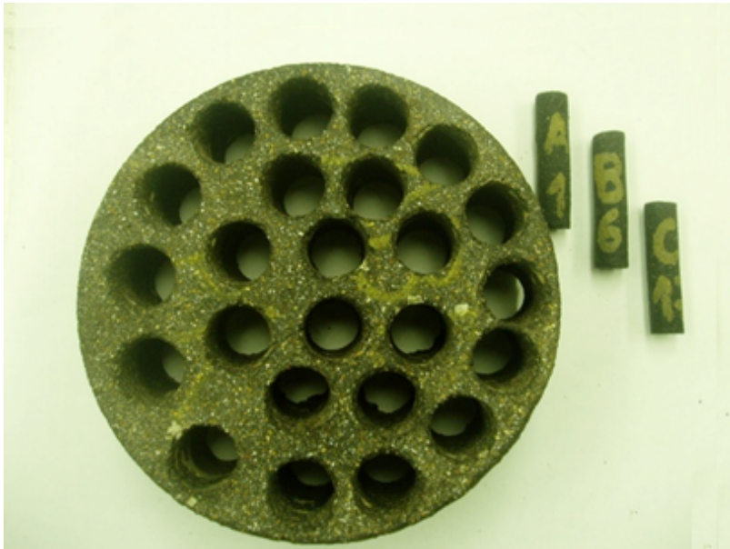
Figure 4.1. Typical FAM Test Specimens Cored Out of a Superpave Gyratory Compacted Specimen
