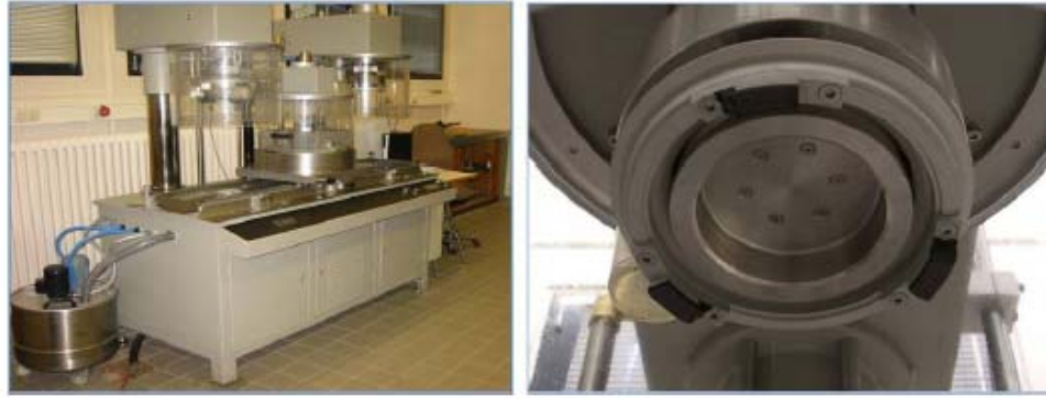
Figure 4.14: Wehner/Schulze device (a) overall view and (b) skid resistance measuring unit (Ueckermann et al., 2014).
