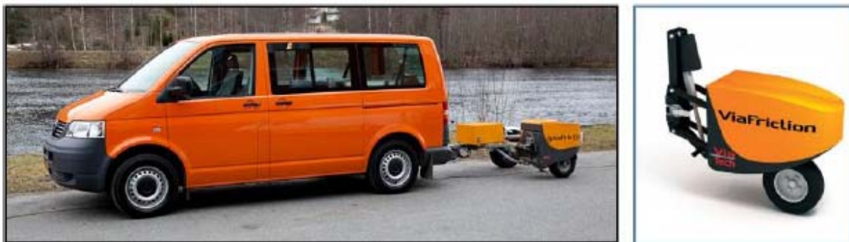
Figure 4.15: Via Friction device (a) overall view and (b) ViaFriction measuring unit (Ueckermann et al., 2014).
