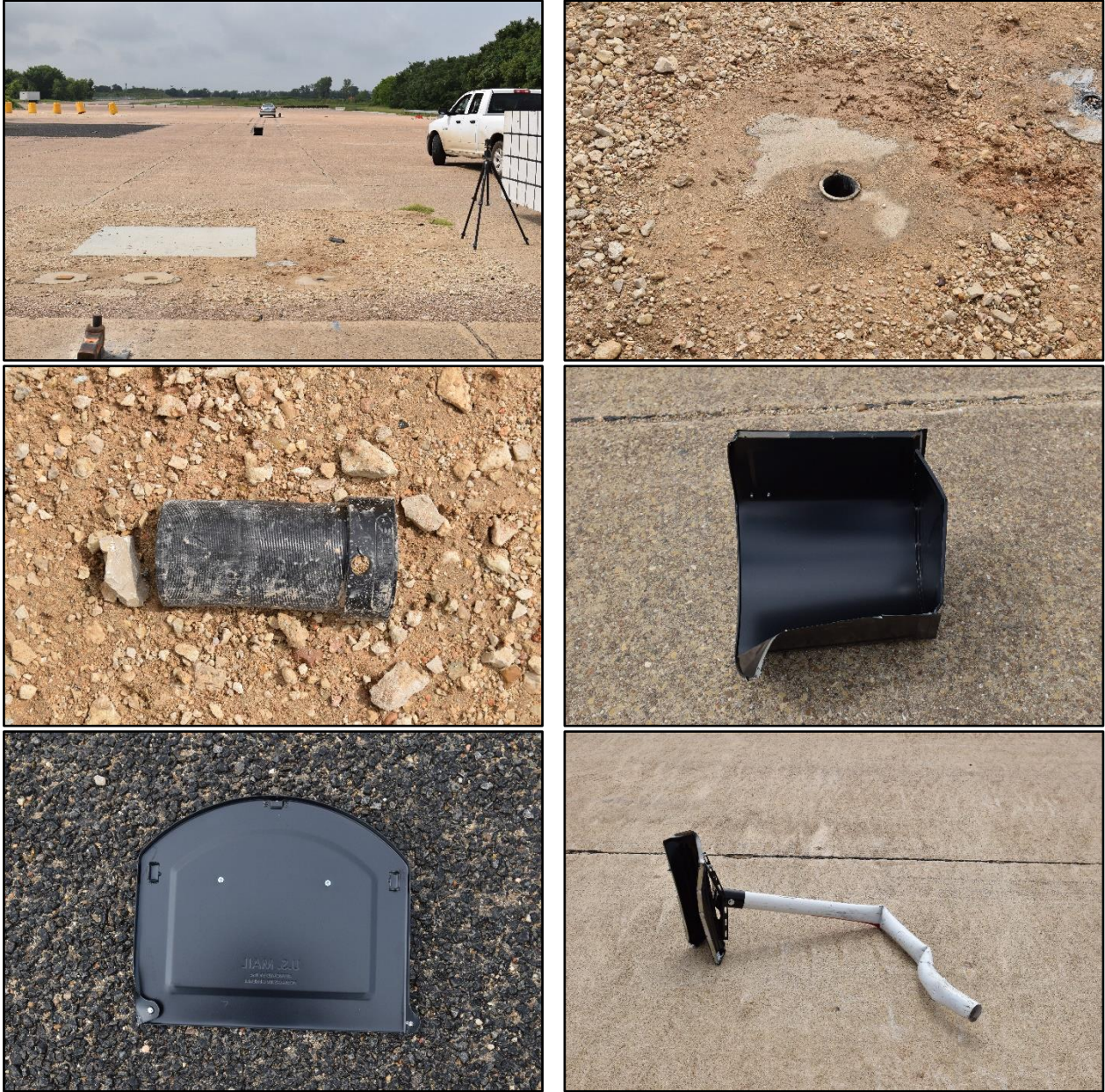
Figure 4.6. Mailbox after Test No. 469689-1-1.
