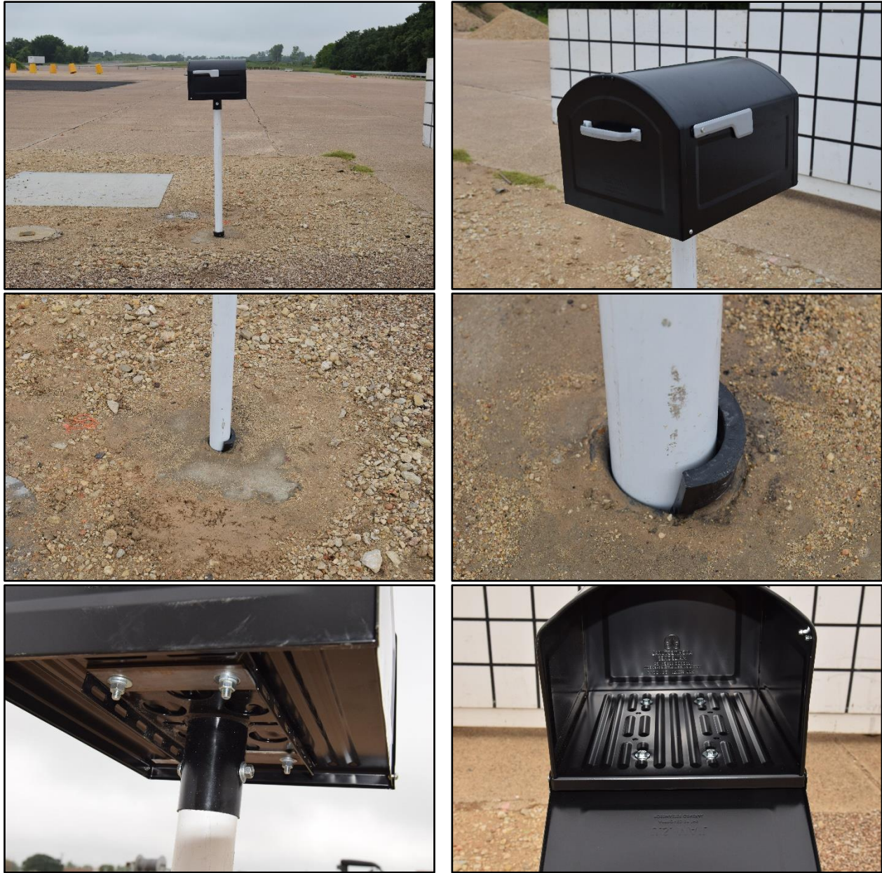
Figure 4.3. Centennial Model Extra-Large Mailbox on Type 4 Support prior to Testing.
