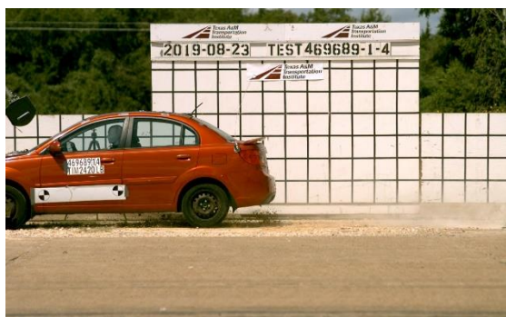
Figure D.1. Sequential Photographs for Test No. 469689-1-4 (Perpendicular and Oblique Views).
