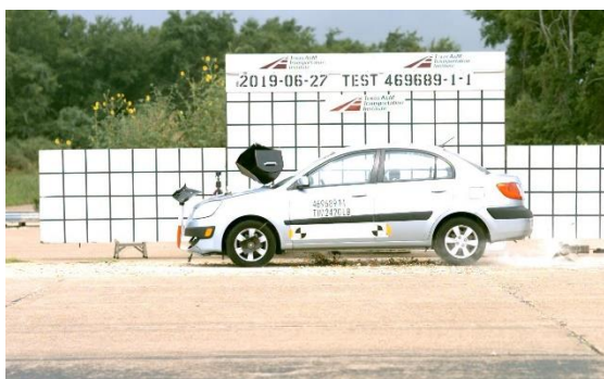
Figure A.1. Sequential Photographs for Test No. 469689-1-1 (Perpendicular and Oblique Views).
