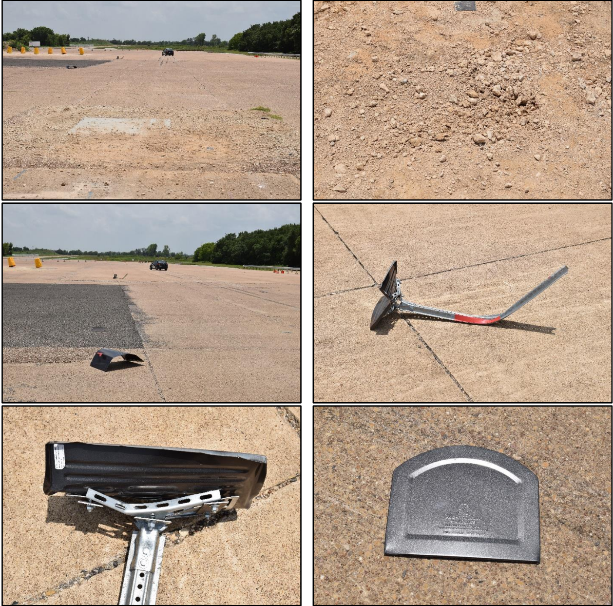
Figure 6.6. Mailbox after Test No. 469689-1-3.
