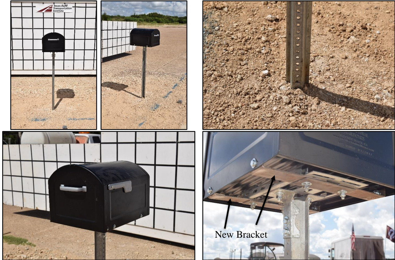
Figure 7.3. Centennial Model Extra-Large Mailbox on Type 3 Support prior to Testing.
