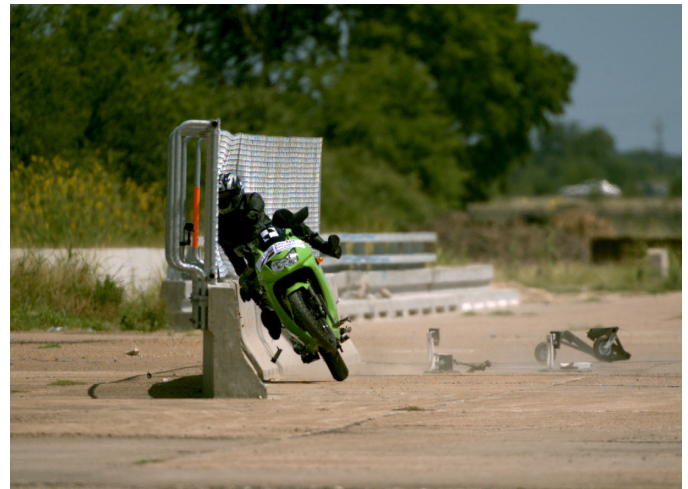
Figure 1. Concrete Barrier-Mounted Containment System for Motorcycle Riders.
