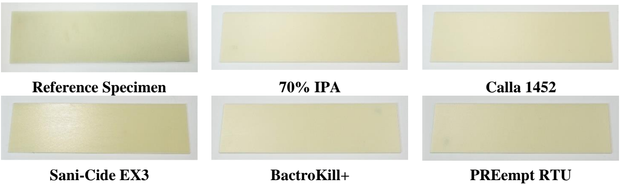
Figure 54. Color qualitative comparison of Fiberglass G-10/FR4
