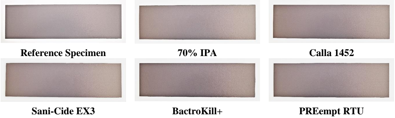
Figure 47. Color qualitative comparison of Aerform LHR
