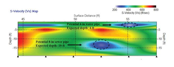
Source: FHWA. (created using MASW ParkSEIS  $\bigcirc$  version 1.01 (Park Seismic LLC. n.d.)). Vs = shear velocity.
