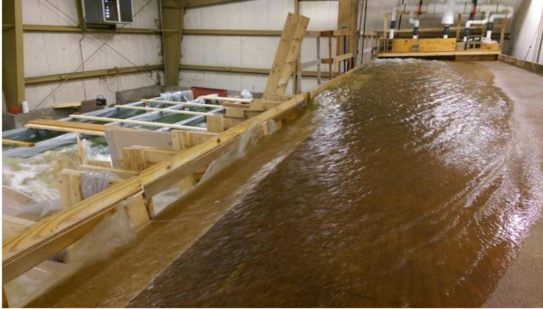
Figure 30: Waves around both internal slab supports for a 15 ft curb inlet (Test#60 in Appendix B).
