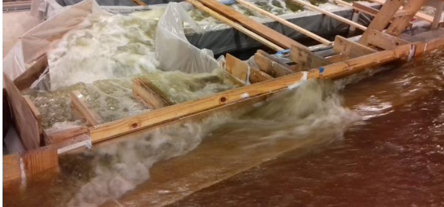
Figure 79: Inflow into the upstream extension being diverted into the main bay (Level A setup).
