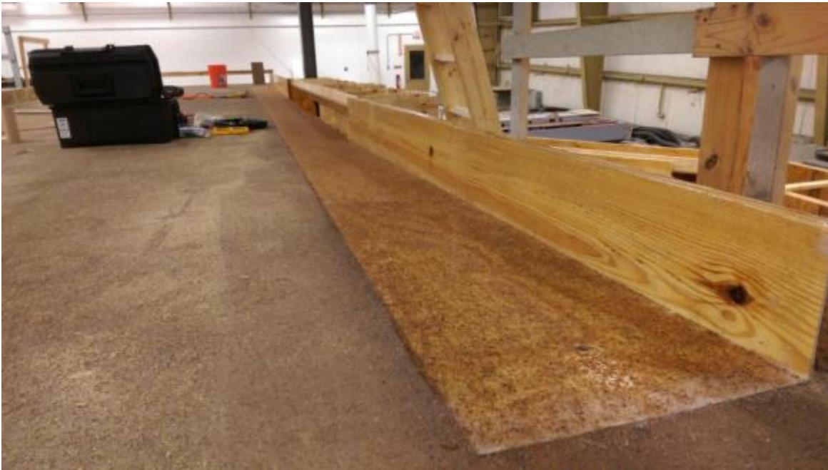
Figure 16: Upstream curb and gutter transition for the full-scale model of conventional curb inlet.
