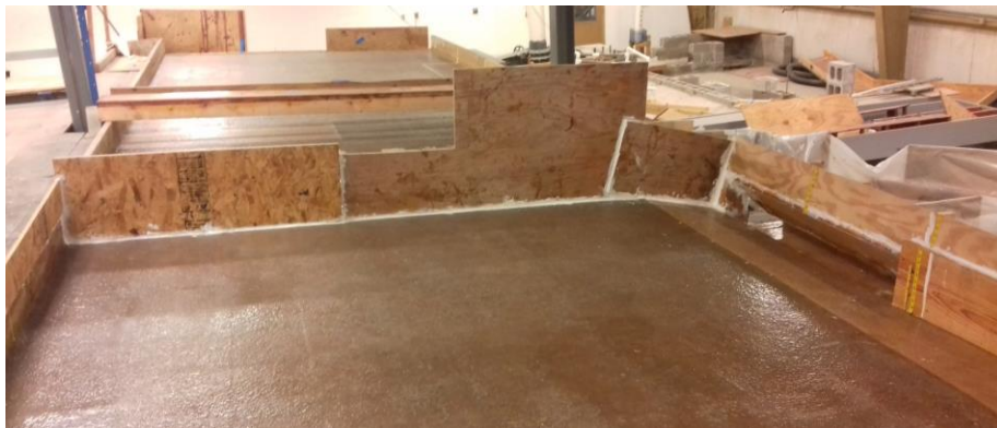
Figure 80: The set-up for the fully-submerged inlet, looking downstream.
