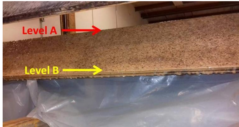
Figure 75: The two tested tail water levels, looking from inside the inlet.
