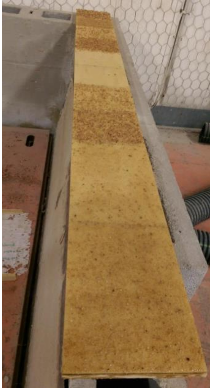
Figure 21: Graded sand variations test panel for matching existing roadway texture.
