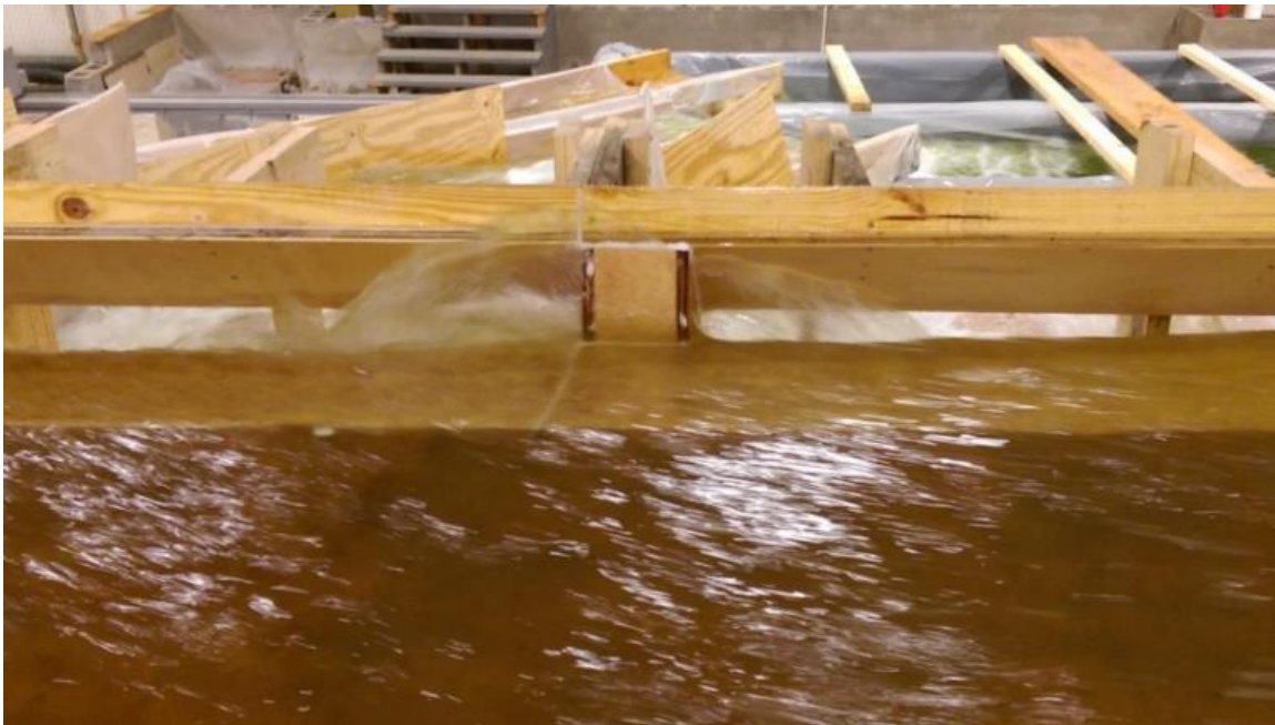
Figure 29: Waves at an internal slab support for a 15 ft curb inlet (Test #60 in Appendix B).
