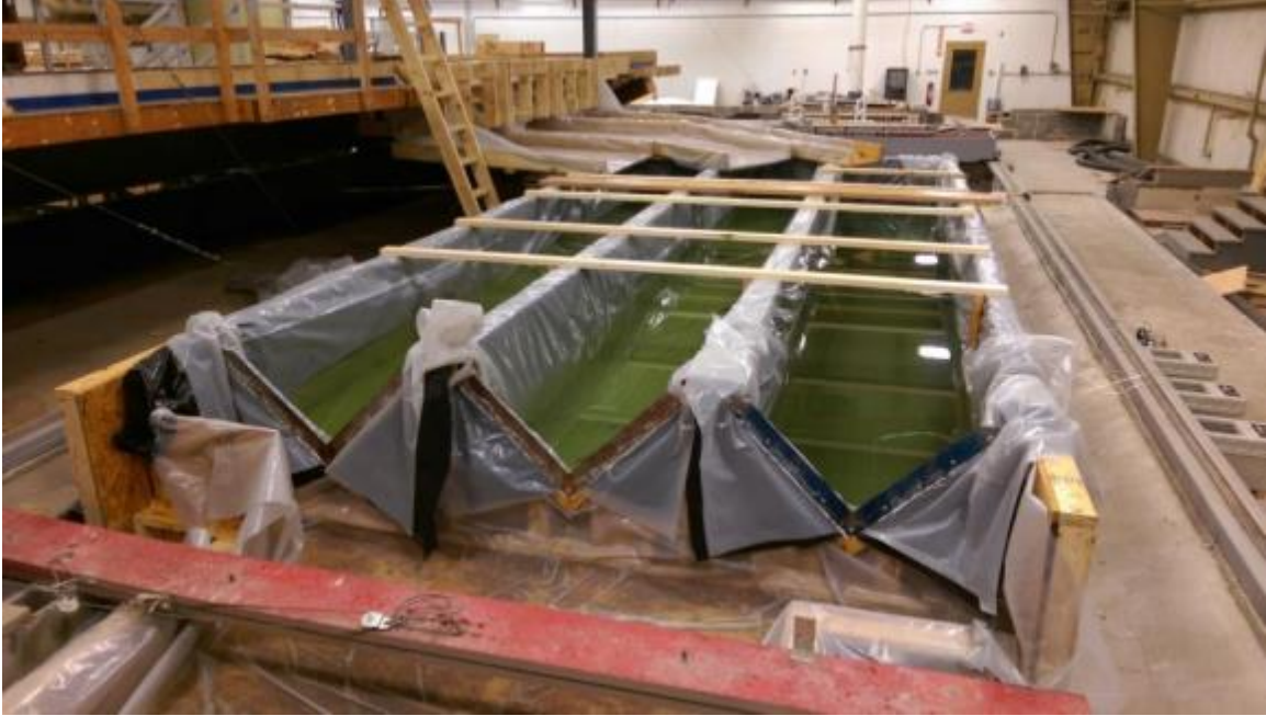
Figure 17: V-notch weirs and approach channels designed for measurement of interception in each bay of conventional 15 ft curb inlet.
