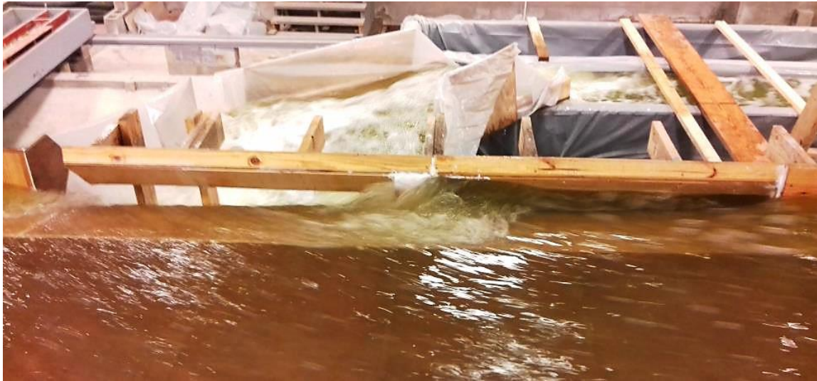
Figure 73: Excess inflow being diverted from the upstream extension to the main inlet section.
