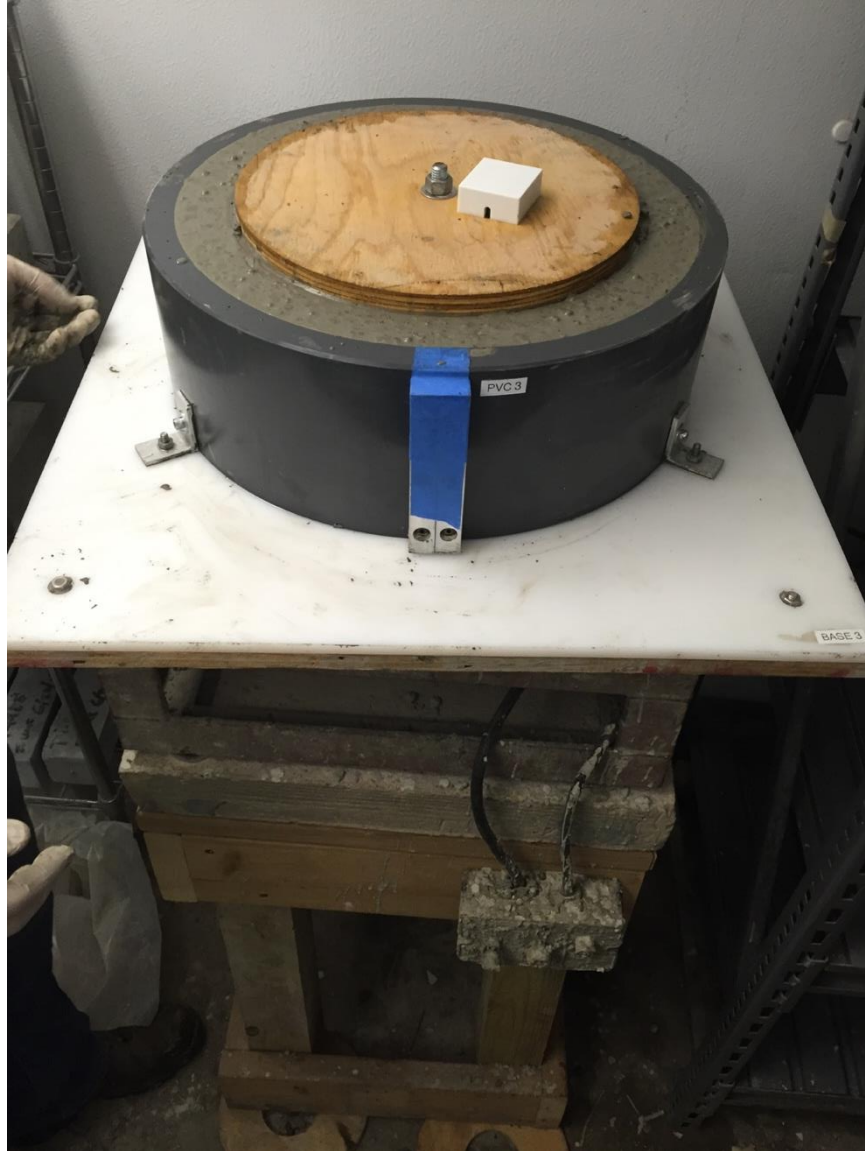
Figure 5-8: Casting restrained shrinkage ring on vibrating table
