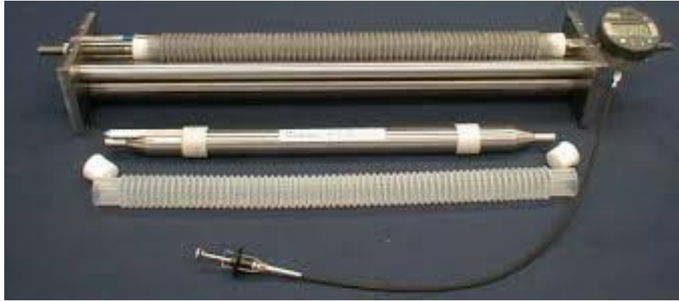
Figure 5-32: Corrugated polyethylene autogenous test setup (Germann Instruments)
