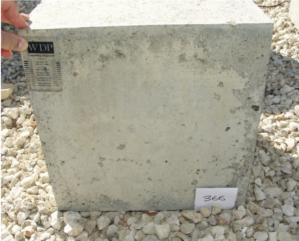
Figure 6-1: Example of Crack Rating = 0
