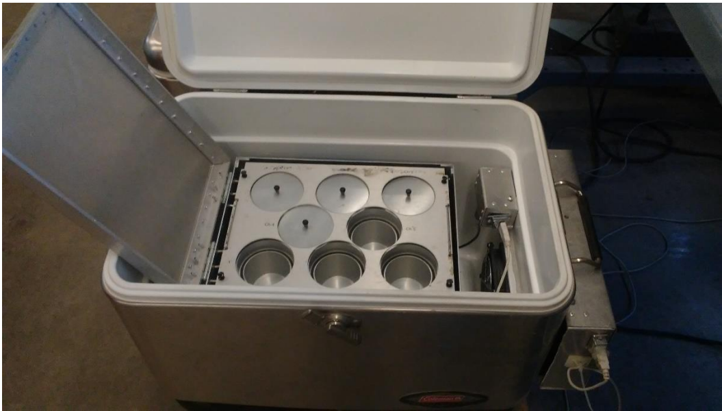
Figure 5-51: Isothermal calorimetry apparatus
