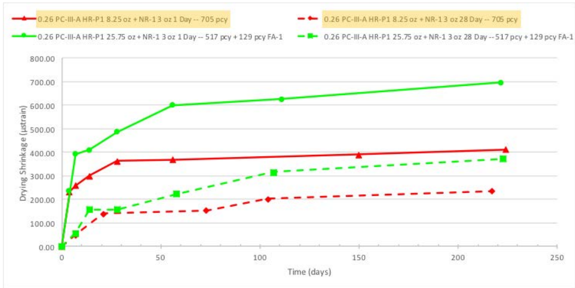
Figure 4-13: Drying shrinkage curve showing effect of cement content for base mixture M1-NC.
