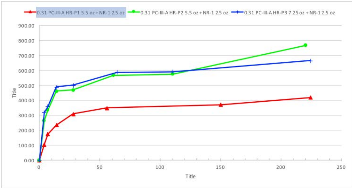
Figure 4-12: Drying shrinkage curve showing effect of HRWR type (HR-P1, HR-P2, and HR-P3) for base mixture M4-SCC.
