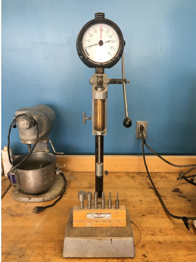
Figure 4-3: Time of set equipment used throughout this project
