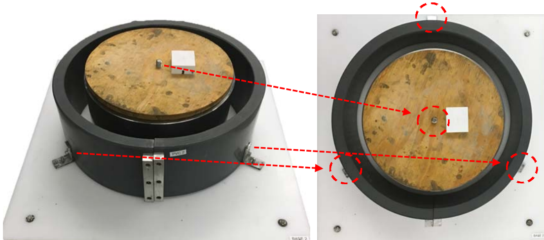
Figure 5-3: Locking locations for securing the inner and outer rings to the restrained shrinkage ring bases denoted in red
