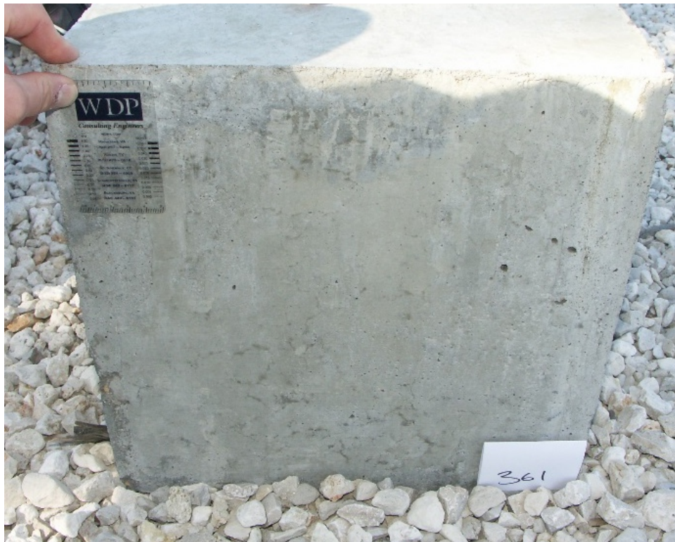
Figure 6-3: Example of Crack Rating = 2
