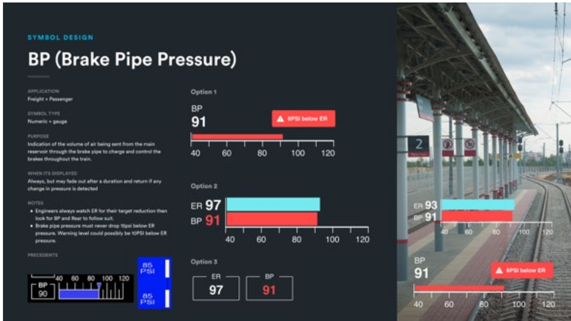
Figure 36: Draft of Brake Pipe (BP) Pressure
