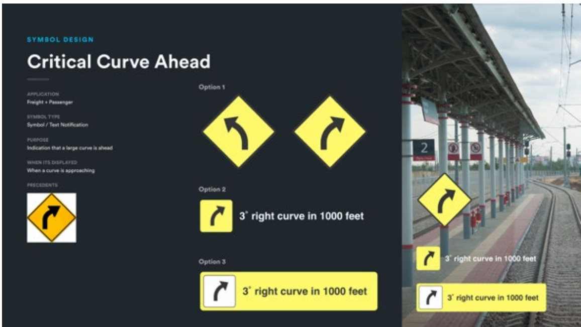
Figure 51: Draft of Critical Curve Ahead
