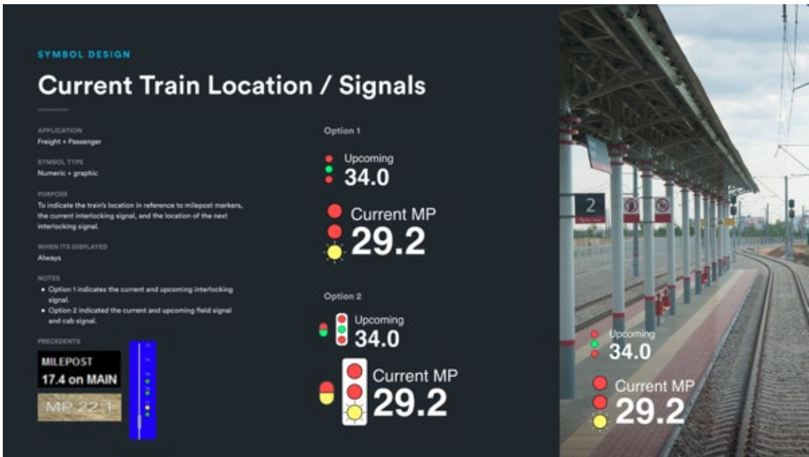
Figure 28: Draft of Current Train Location/Signals
