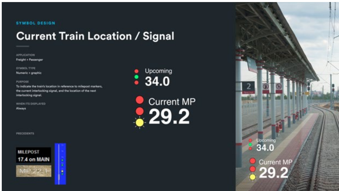
Figure 86: Task 5 Final Symbol for Current Train Location/Signal
