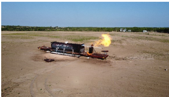
Figure 4. Test in Progress – PRV Operating (After Fire Source Burner Turned Off)
