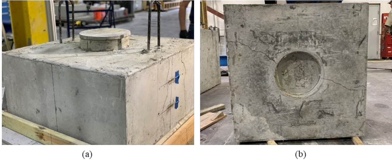
Figure A.24: Cracking on the (a) east side and (b) bottom of Specimen S2-1
