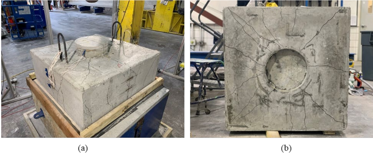
Figure A.52: Cracking on a (a) cap and (b) bottom of the Specimen S2-5
