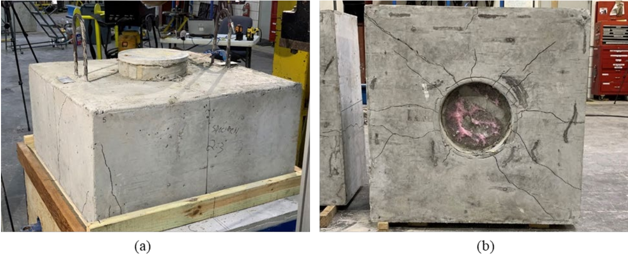
Figure A.38: Cracking on (a) cap and (b) bottom of the Specimen S2-3
