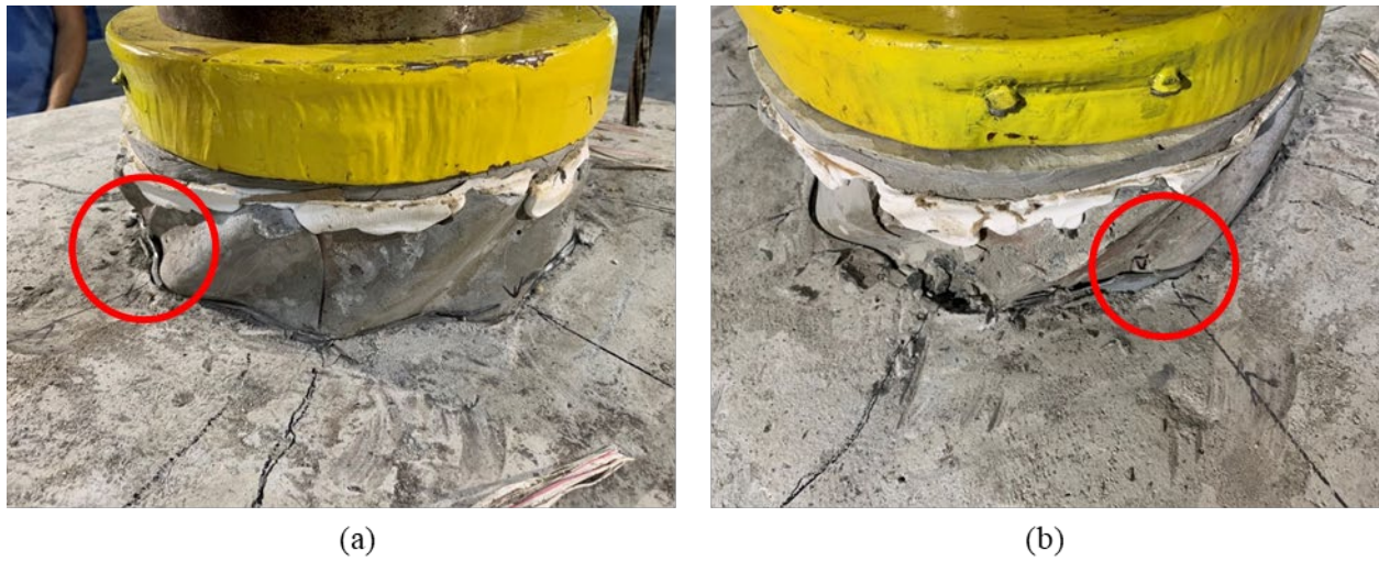
Figure A.82: Details of plug rotation in (a) separation of the interface is observed and in (b) reference lines do not match
