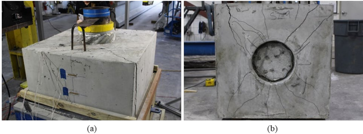
Figure A.80: Cracking on (a) cap and (b) bottom of Specimen S2-9
