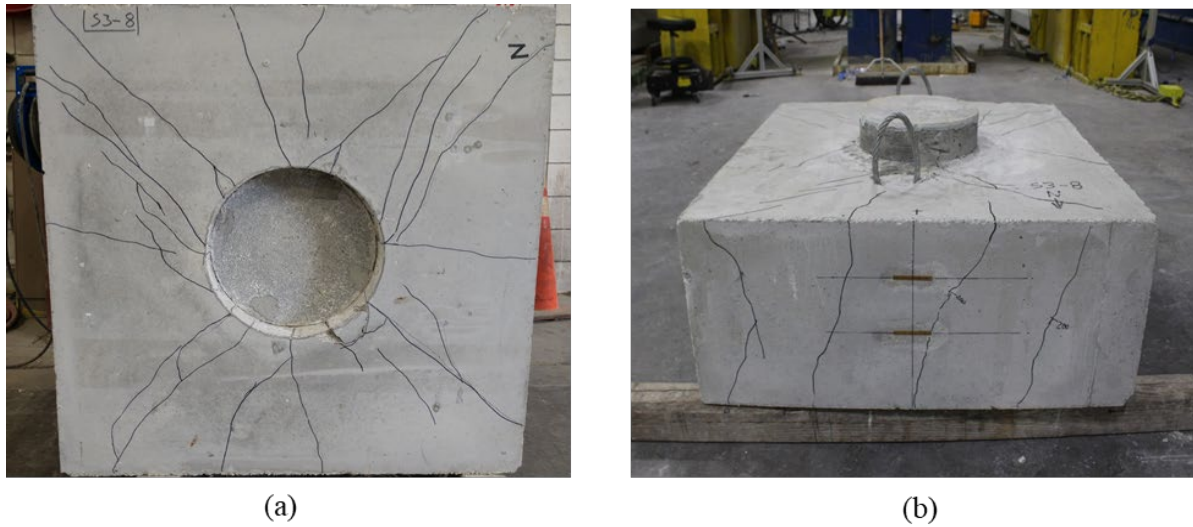
Figure A.190: Cracking on (a) bottom and (b) cap of Specimen S3-8
