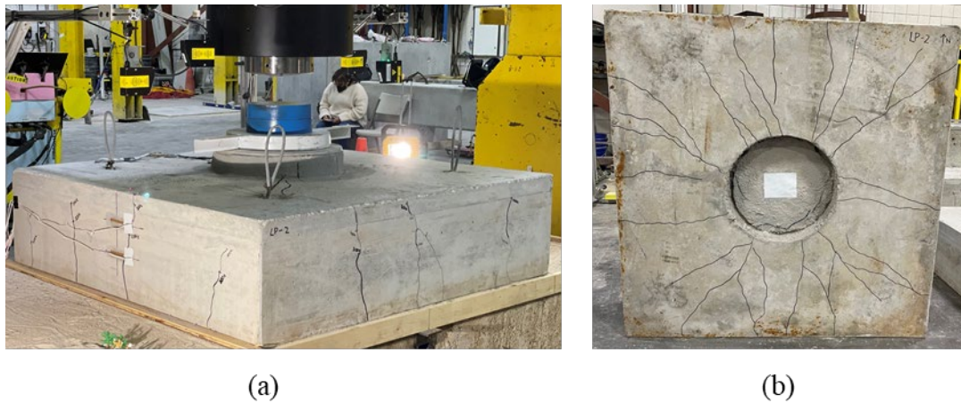
Figure B.14: Cracking after testing on (a) south-west side and (b) bottom of the Specimen LP-2
