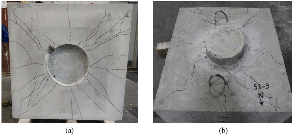
Figure A.156: Cracking after testing on (a) bottom of the cap and (b) top of the cap of Specimen S3-3
