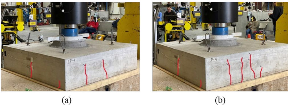
Figure B.24: Crack propagation during testing at (a) 200 kips and (b) 300 kips
