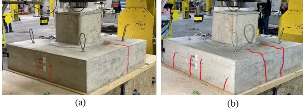
Figure B.54: Crack pattern at (a) 175 kips and (b) 350 kips for SC-2
