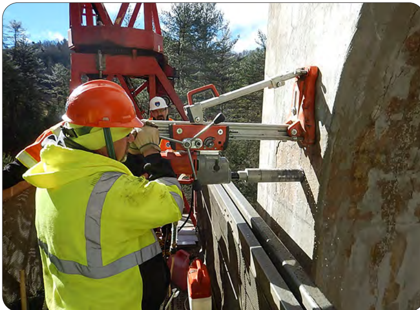
EFLHD Bridge Inspection Team perform core sampling (left) and structural review (above) — Laurel Fork Bridge, Blue Ridge Parkway, North Carolina
