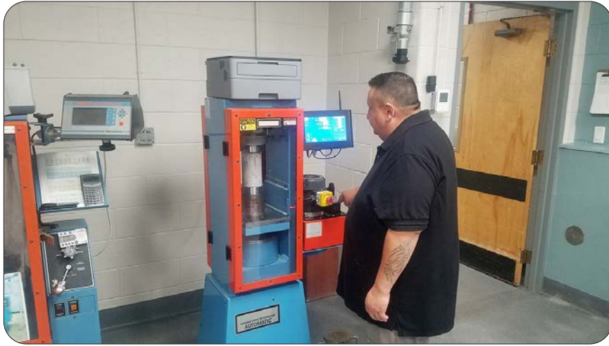
Chris Garcia, CFLHD Materials Engineering Technician breaking a concrete cylinder on a new 400,000 lb. press. — Lakewood, Colorado
