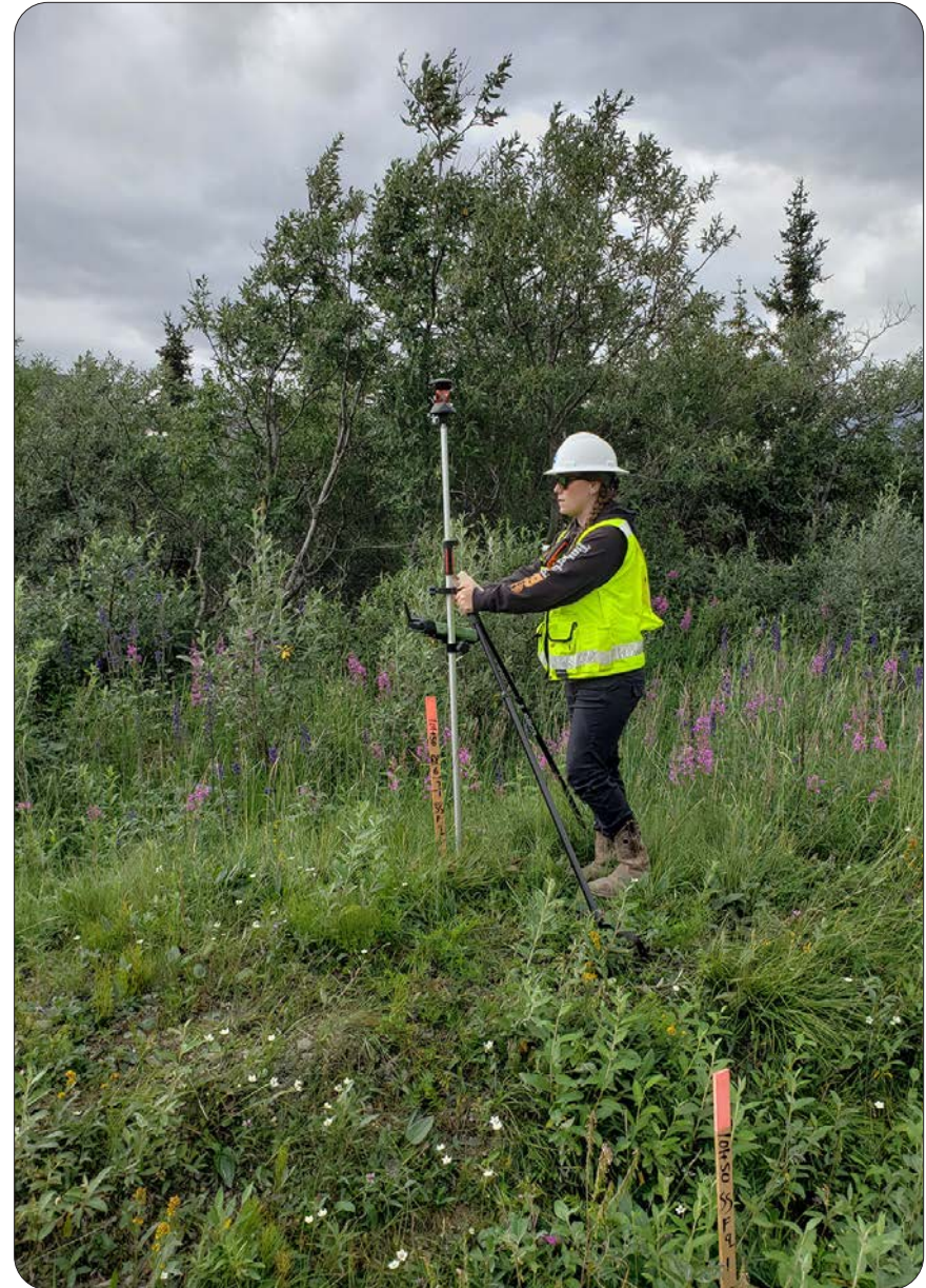
WFLHD Assistant Project Engineer, Renee Newman checks staking — Denali National Park, Alaska
