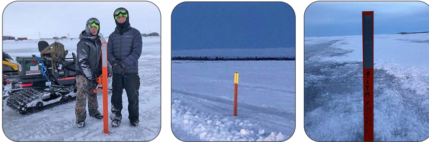
A first for the Kuskokwim Ice Road – standardized markers provided by Alaska DOT, amber reflectors face downstream, silver reflectors face upstream — Alaska
