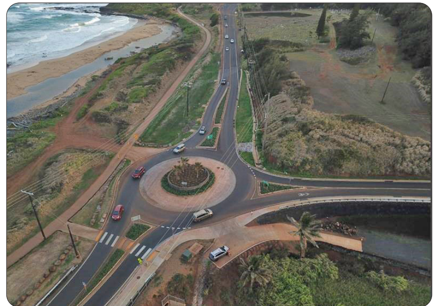
Kapaa Stream Bridge and Mailihuna Road intersection rehab and safety improvements projects (above & below) addressed bridge width, load capacity, bridge railing and transitions, and bridge approaches. The highway intersection at Mailihuna Road was also improved with lighting, signing, pavement marking, drainage, traffic signal installation, roadway widening and other improvements. — Island of Kauai, Hawaii
