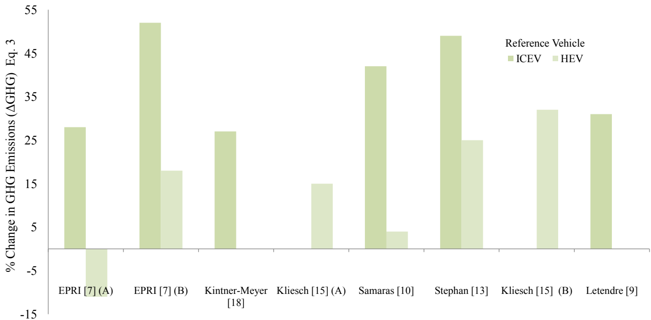
Figure 1-2. Change in GHG Emissions. [7] (A) assumed charging with electricity generated from coal power plants while [7] (B) assumed that the electricity was generated from combined cycle natural gas. [18], [15] (A), [10] and [13] all used the national average generating mix while [15] (B) & [9] used regional averages for CA and New England respectively.
